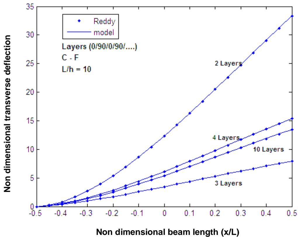
Figure (8) a: **Non dimensional** transverse deflection of cantilever composite beam.
