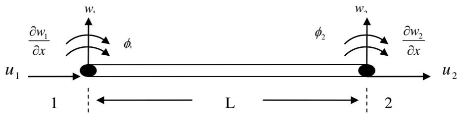
Figure (2): Degrees of freedom at each node of the beam element
