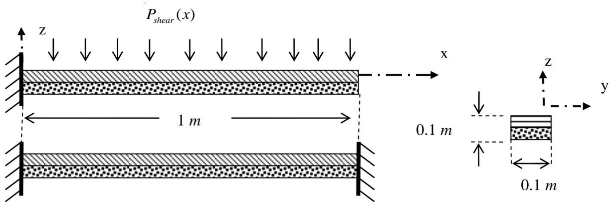
Figure (6): Geometric characteristics of C-F and C-C composite beams
