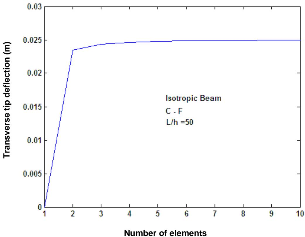
Figure (4): Effect of the number of elements on the transverse deflection
