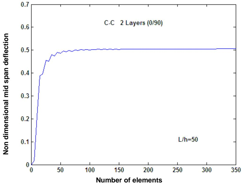
Figure (7) b: Effect of the number of element on mid span deflection of clamped-clamped beam.
