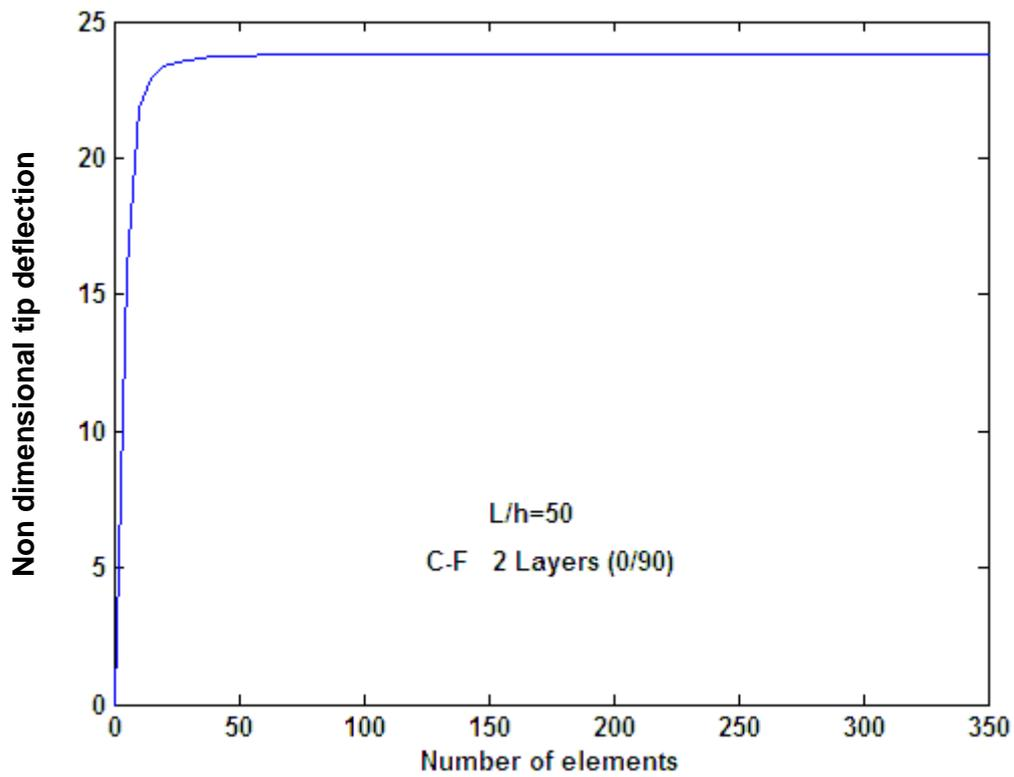
Figure (7) a: Effect of the number of element on tip deflection of clamped-free beam.
