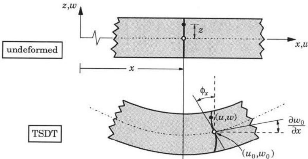
Figure (1): Un-deformed and Deformed cross section [10]
