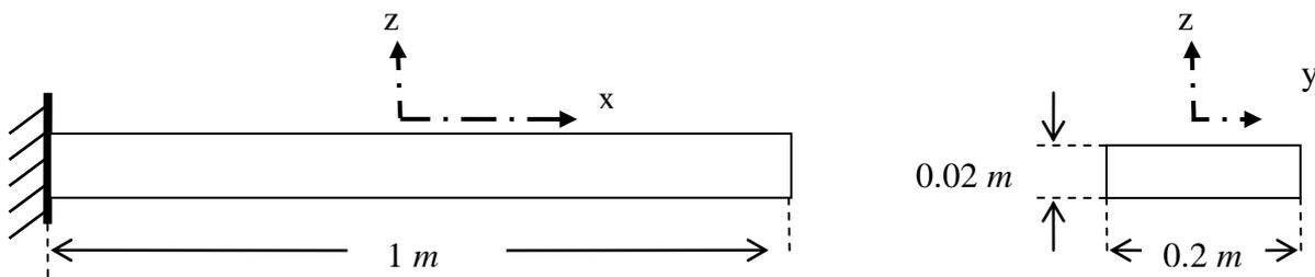
Figure (3): An isotropic cantilever beam
