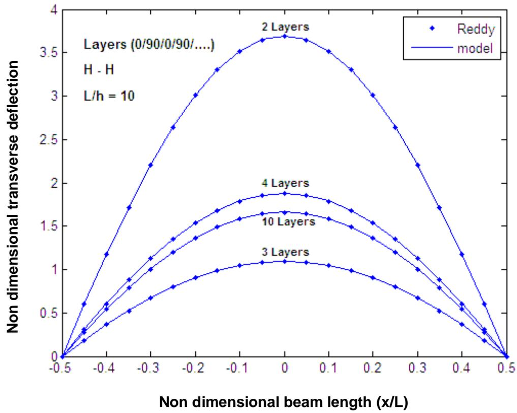
Figure (8) b: Non dimensional transverse deflection of hinged-hinged composite beam.
