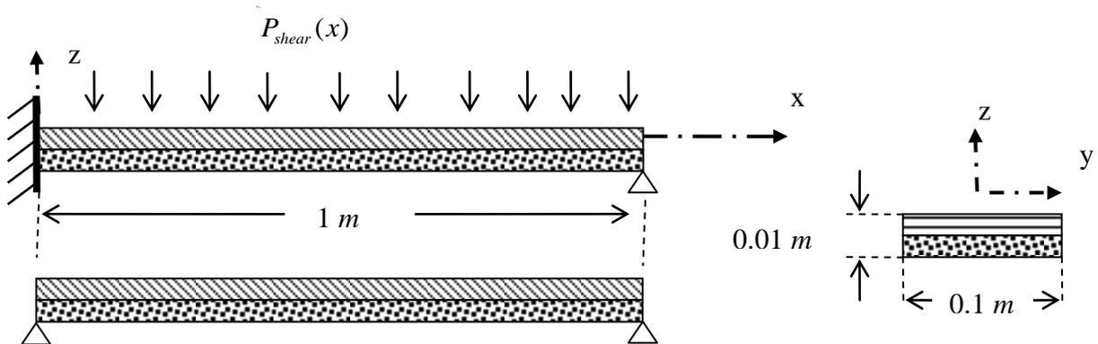
Figure (9): Geometry of C-H and H-H composite beams
