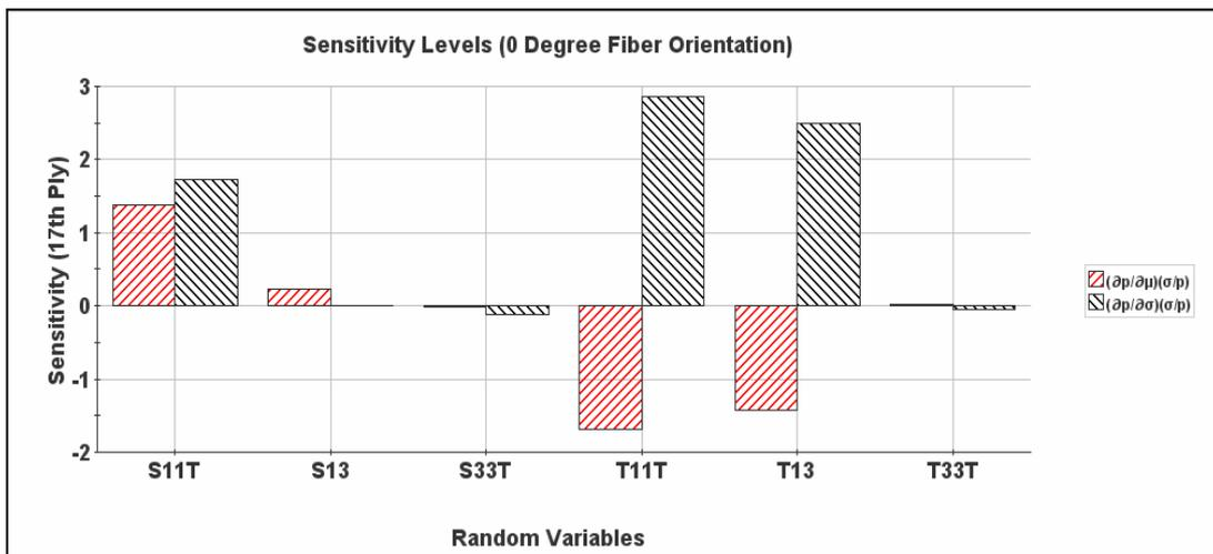
Fig. 5. Sensitivity analysis of random variables at 0° fiber orientation.
