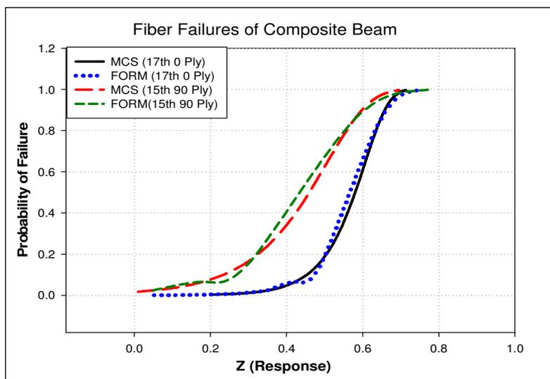
**Fig. 3.** Comparison of probability of fiber failures at Monte Carlo Simulation (MCS) and first order reliability method (FORM).
