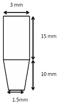
**Fig.1.** Impactor Geometry.
