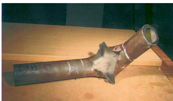
Fig. 28. Ductile 'cobra hood' rupture in an economizer tube.
