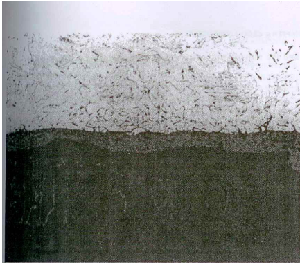
Fig. 2(a). Tightly bound ID scale, 25x.
