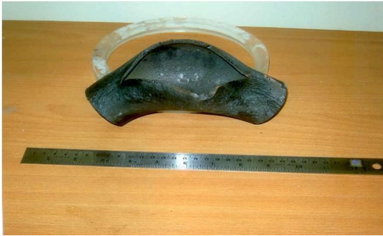
Fig. 21. 'Fish mouth' ruptures of a reheat tube due to grain growth and creep deformation.
