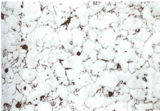
Fig. 9. Spheroidized iron carbide dispersed in matrix and onset of graphitization.
