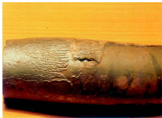
Fig.12. Slit formation in an economizer tube due to graphitization.
