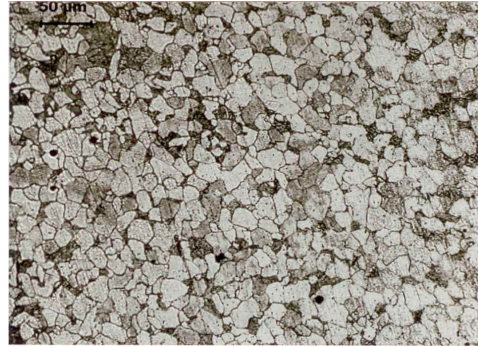
Fig. 22 (a). Normal ferrite-pearlite structure in the unaffected portion, 200x.
