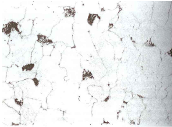
Fig. 7. Normalized ferrite-pearlite structure in SA-178 steel, 500x.
