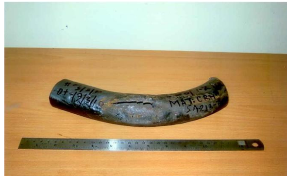
Fig. 14. Thick-lip rupture of a superheater tube due to graphitization.
