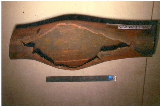
Fig. 24. A 'fish mouth' rupture of a waterwall tube due to hydrogen damage.
