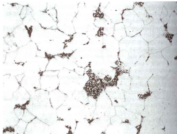
Fig. 8. In-situ spheroidization of pearlite in still well defined colonies, 500x.
