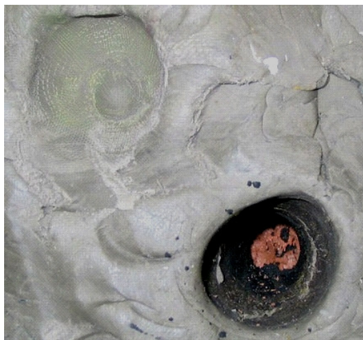
Fig.1. Perforation of IIIA type body armor by next test bullet in distance about 20% closer than required by standard.
