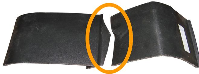
**Fig. 11.** Broken specimen (tested with filling material double layer of carton as a honey comb)
