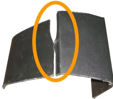
**Fig. 9.** Broken specimen(tested without filling material)
