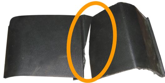
**Fig. 10.** Broken specimen( tested with filling material -sponge 30 in intensity)
