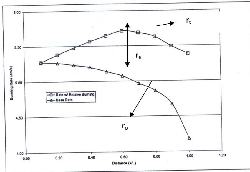
**Fig. 2.** Erosive burning rate compared to base rate [3].
