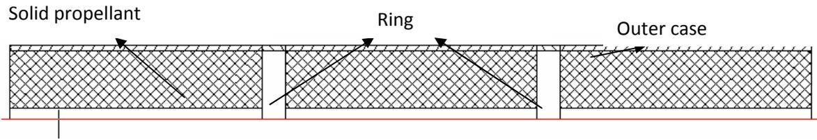
**Fig. 10.** Segmented propellants in rocket motor.
