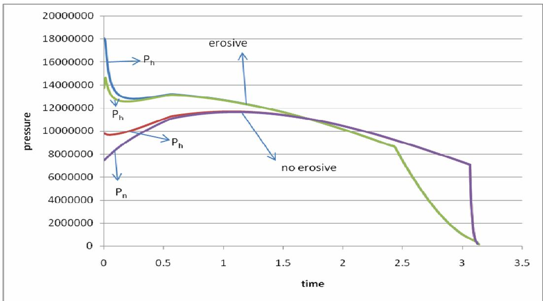
**Fig. 15.** Pressure time curve with and without erosive burning.
