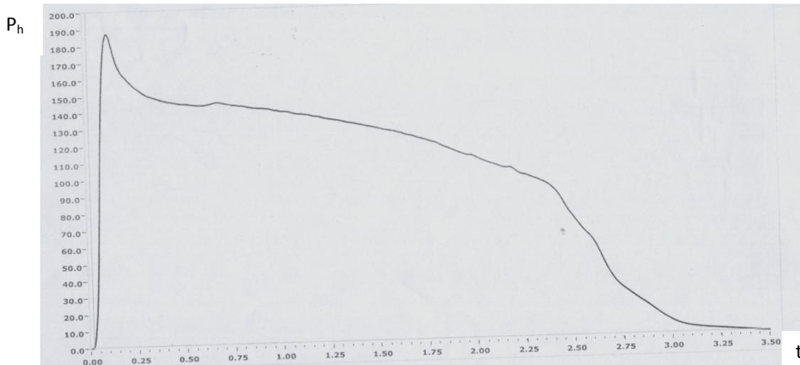
**Fig. 11.** Pressure time curve of type 3 of propellant.
