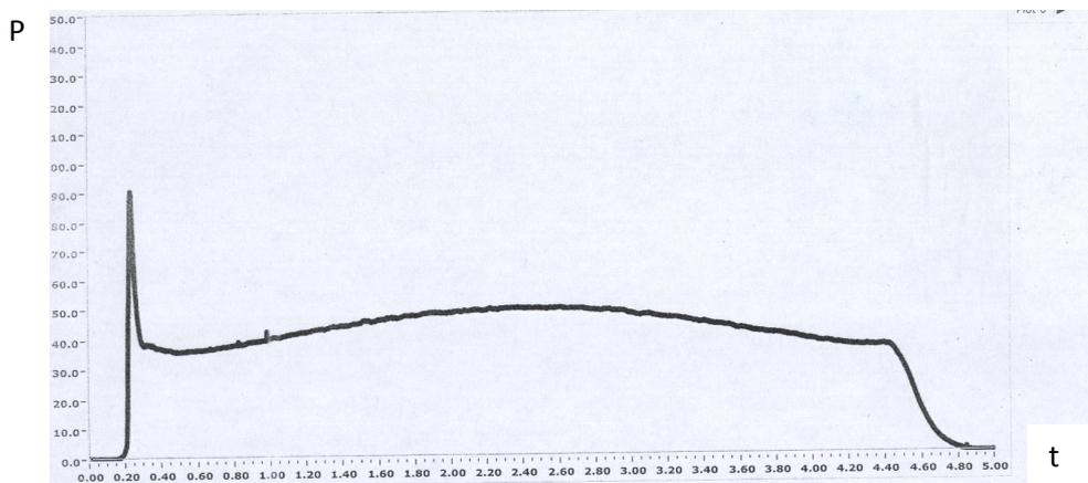
**Fig. 5.** Pressure time curve at port diameter 10 mm.
