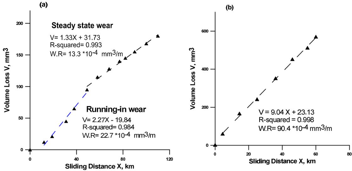
Fig. 2. Variation of PA66 volume loss with sliding distance at 90 N applied load (a) dry and (b) wet.
