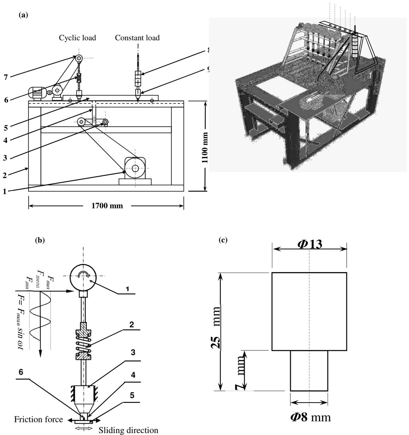
**Fig. 1.** (a) Tribometer; (1) motor; (2) machine frame; (3) chain drive mechanism; (4) U-beam guide; (5) reciprocating carriage; (6) spring; (7) eccentric cam; (8) dead weights; (9) pin holder.
