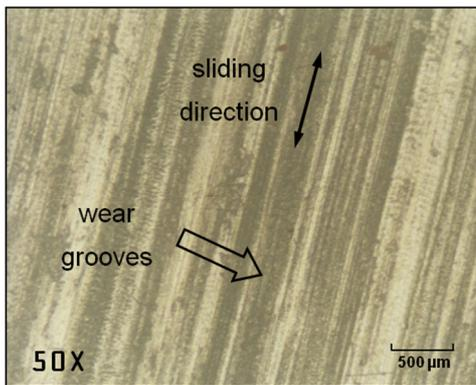
Fig. 3. PA 66 worn surface after 80 km of sliding,  $F=90 \text{ N}$ .
