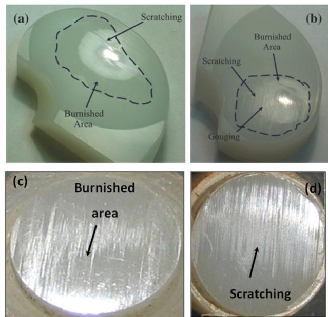
Fig. 8. (a, b) worn/burnished areas and some slight scratching and gouging of UHMWPE tested in orthopedic wear simulator, adopted from Ref. [14], (c, d) scratching and burnished area of wear surfaces of PA66 ( $F_{mean} = 90\text{N}$ ,  $f = 1.5 \text{ Hz}$ ).
