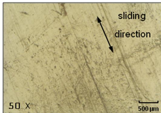
Fig. 4. PA 66 worn surface after 40 km sliding distance, at 90 N applied load.
