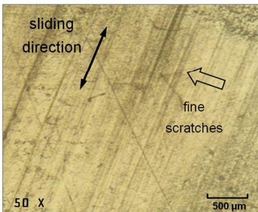
Fig. 7. PA 66 worn surface after 40 km sliding distance ( $F_{mean} = 90\text{N}$ ,  $f = 1.5 \text{ Hz}$ ).
