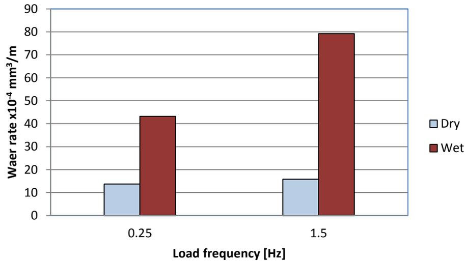
Fig. 6. Variation of PA66 wear rate WR with cyclic load in dry and water-lubricated sliding conditions.
