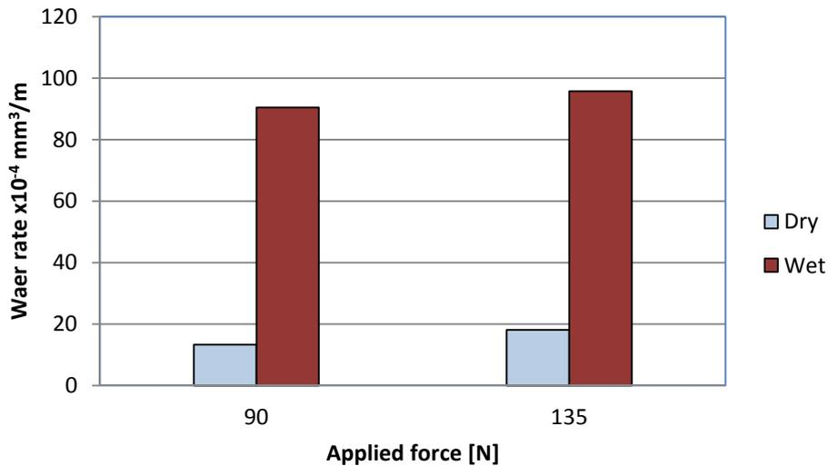
Fig. 5. Variation of PA66 wear rate WR with constant load in dry and water-lubricated sliding conditions.
