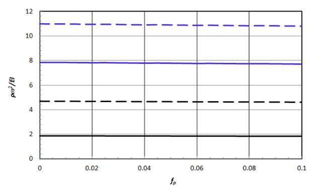
**Fig. 4.** The first four non-dimensional natural frequencies based on Euler theory.
