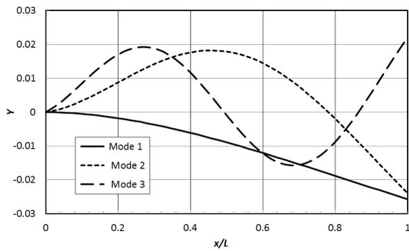
**Fig. 7.** The first three mode shapes based on Timoshenko theory (for extreme values of  $f_p$ ).
