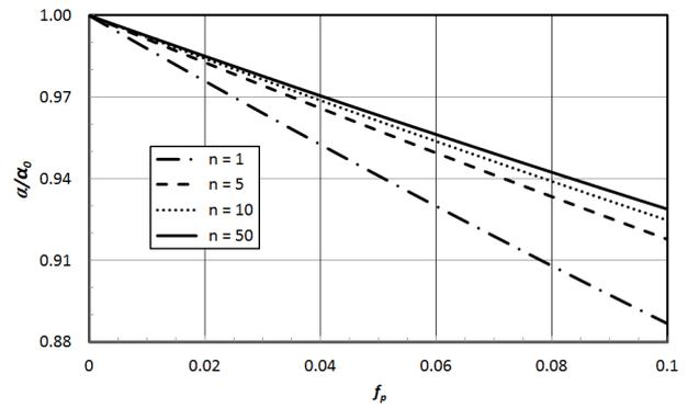
**Fig. 2.** Variation of the NCTE with  $f_p$  for different numbers of layers.
