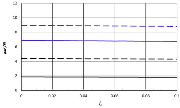
**Fig. 5.** The first four non-dimensional natural frequencies based on Timoshenko theory.
