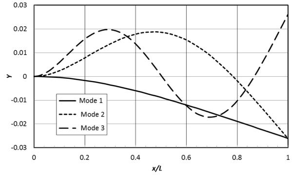
**Fig. 6.** The first three mode shapes based on Euler theory (for extreme values of  $f_p$ ).
