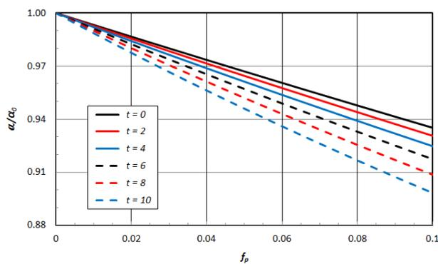
**Fig. 3.** Variation of the normalized CTE with  $f_p$  for different values of the interphase thickness.
