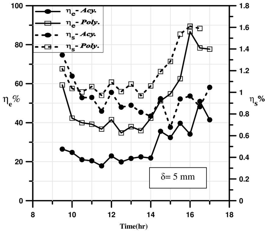
**Fig. 4** Electrolyzer and overall system efficiencies at 5 mm gap distance between the two electrodes.
