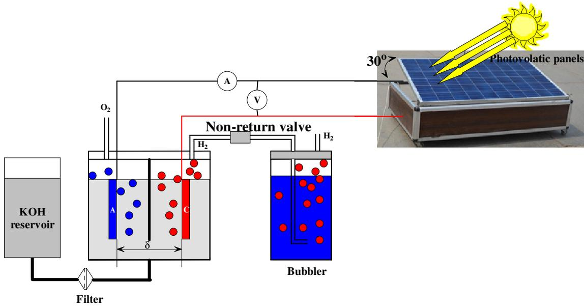
**Fig. 1** Experimental arrangement of the solar hydrogen system.
