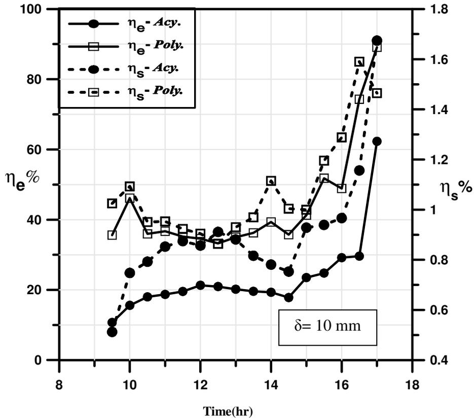
**Fig. 5** Electrolyzer and overall system efficiencies at 10 mm gap distance between the two electrodes.
