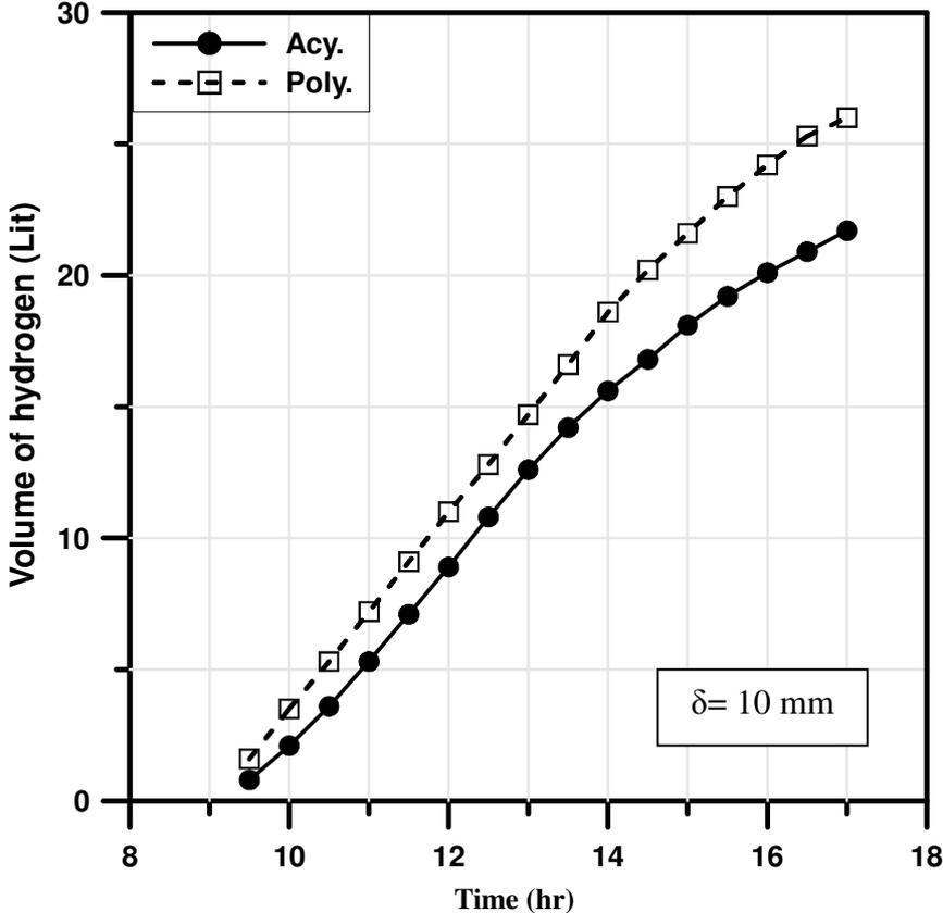
**Fig. 7** Accumulated volume of hydrogen produced through the day time, at 10 mm gap distance between the two electrodes.
