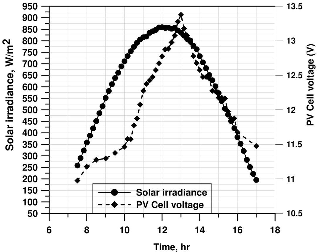
**Fig. 2** Variation of solar irradiance and PV cell voltage through the day time.
