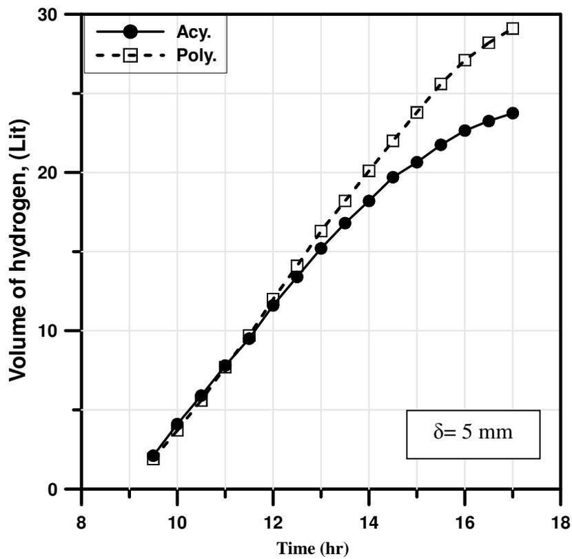
**Fig. 6** Accumulated volume of hydrogen produced through the day time, at 5 mm gap distance between the two electrodes.
