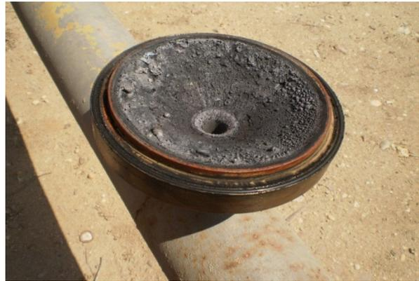
**Fig. 23** Fiber Glass nozzle after the firing test.
