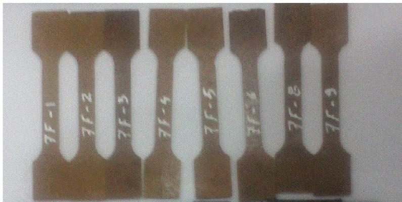
**Fig. 5** JANNAF samples for Fiber Glass / Epoxy.
