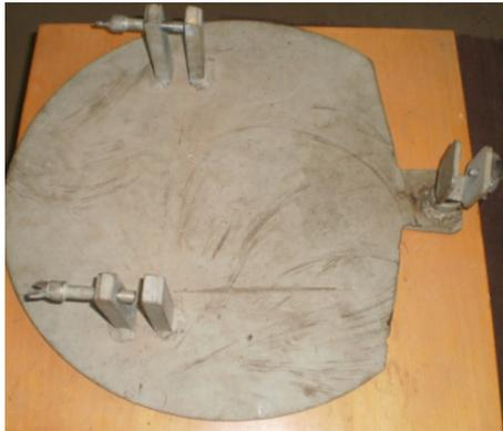
**Fig. 11** Test stand for ablation test.
