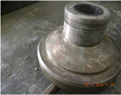
**Fig. 22** Holes in the manufactured nozzle.
