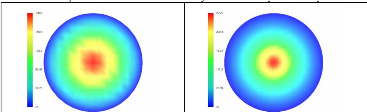
Nd:YVO<sub>4</sub> Crystal with dimension of 0.5\*10mm and central temp. of 188°C
