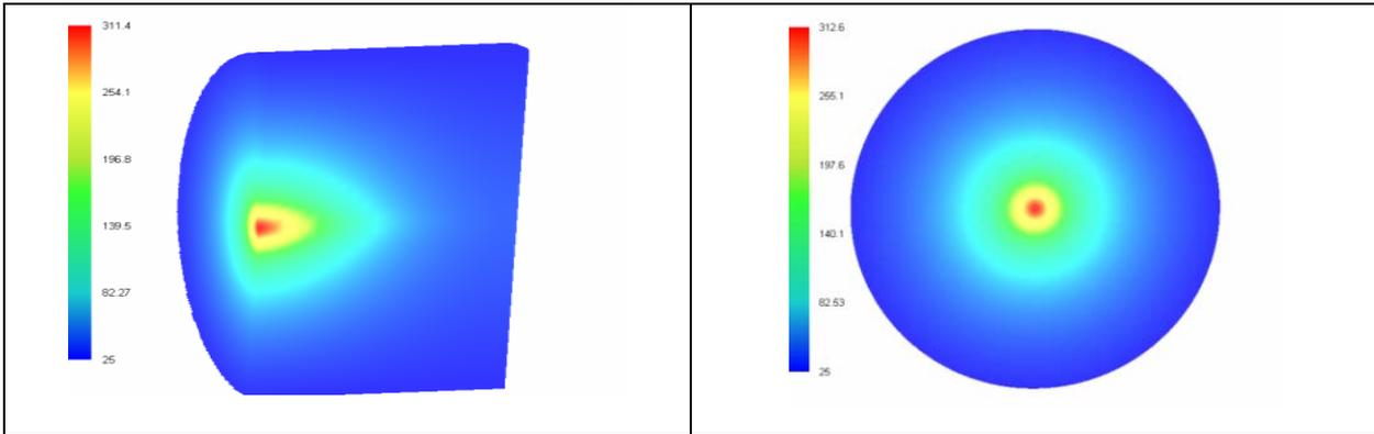
Thermal gradient for 7.8W(focused on the front rod face) pumped 3\*2mm Nd:YVO<sub>4</sub> crystal
