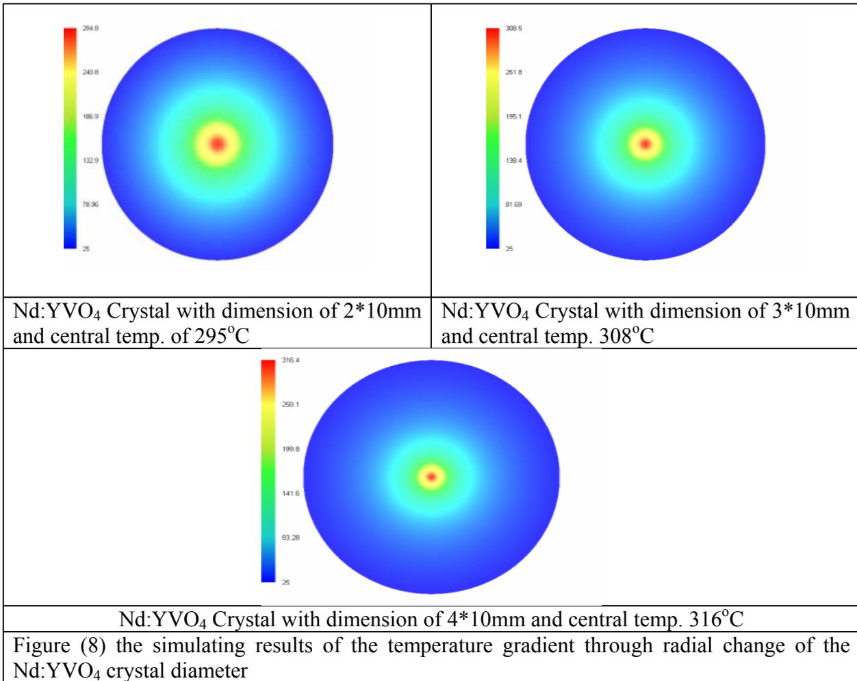
These simulated results manifested the reason of increasing the fracture limit as the crystal diameter became smaller as shown in figure (9).
