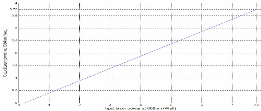
Figure (2) the calculated o/p laser power as a function of i/p laser one.
