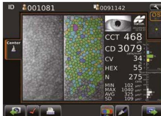
Figure [3]: Showing many marks on the screen as Examine, Mark for print / output, Print, Manual editing, Chinrest up / down, Overlay, Next
