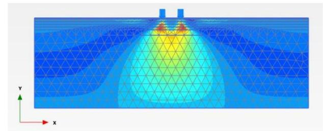
**Figure 5: Lateral strain distribution for S1**
