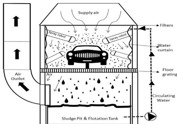
Figure 3: schematic for vehicle coating and VOCs pollutants release
