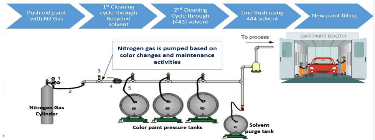
Figure 7 Using layout of Nitrogen gas
