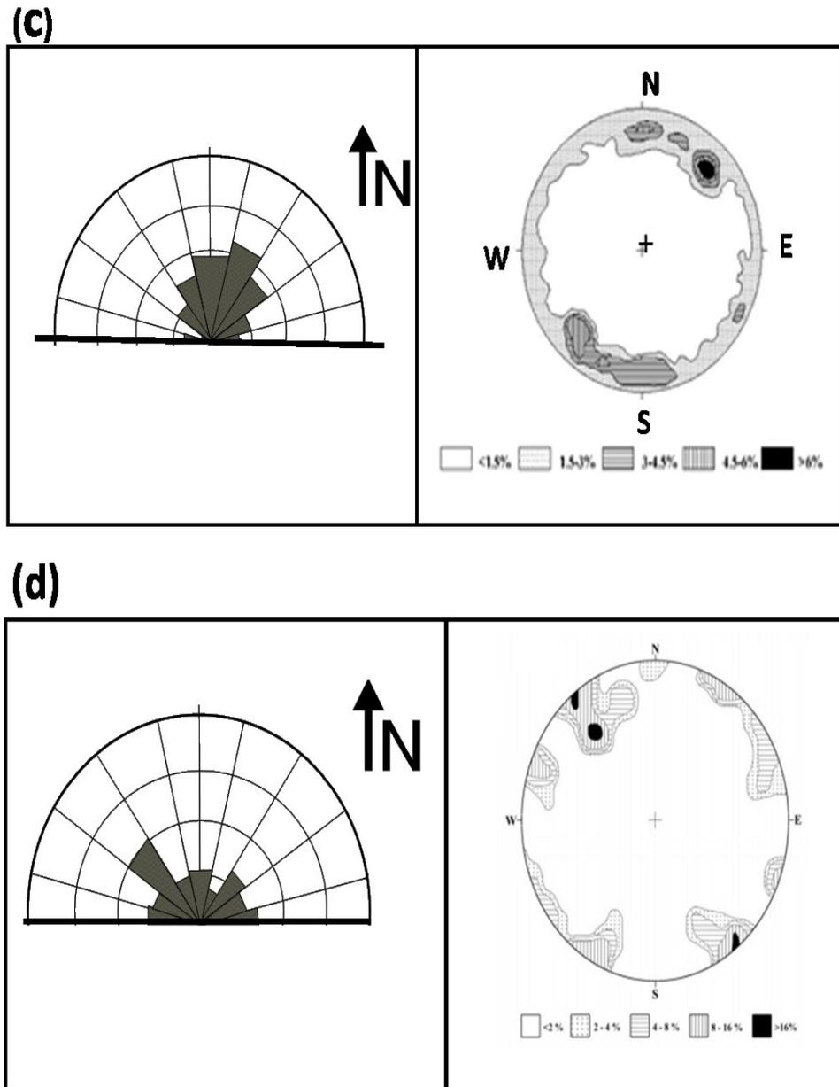
**Fig. 6: Rose diagram and point contour diagram of joints in (a) Dokhan volcanics, (b) Hammamat sedimentary rocks, (c) younger granite rocks (G. Gattar), (d) younger granites (G. Abu Harba).**
