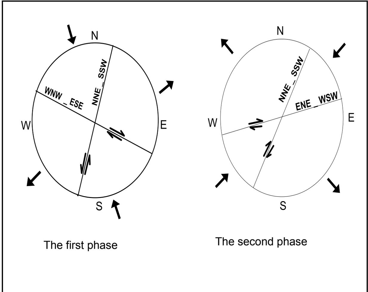
Fig. 5: Stress analysis of the major recorded faults in the study area.
