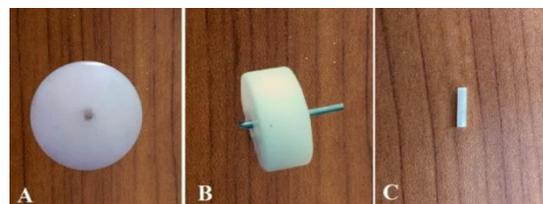
Fig (1): showing (A) and (B) A standardized cylindrical mold, (C) The specimen of composite resin
