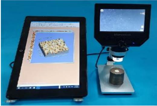
Fig (2): showing a digital microscope with a built-in camera.
