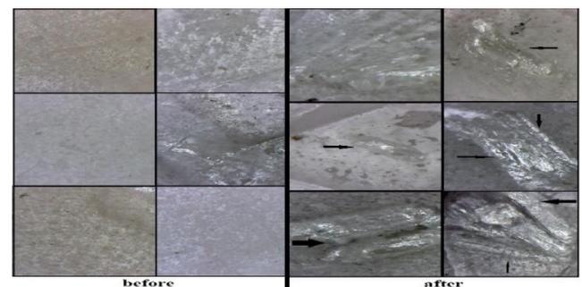
Fig (4): The surface roughness images using USB Digital microscope before and after wear simulation of the 1st group.
