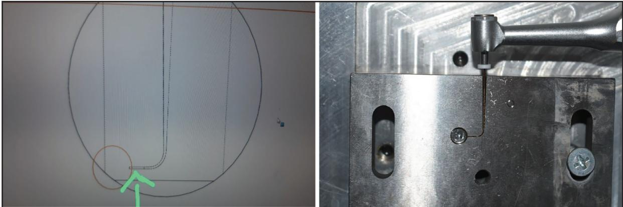
Fig. (1) (1a-b): Artificial 90° stainless-steel canal and motor holder on the metallic board.
