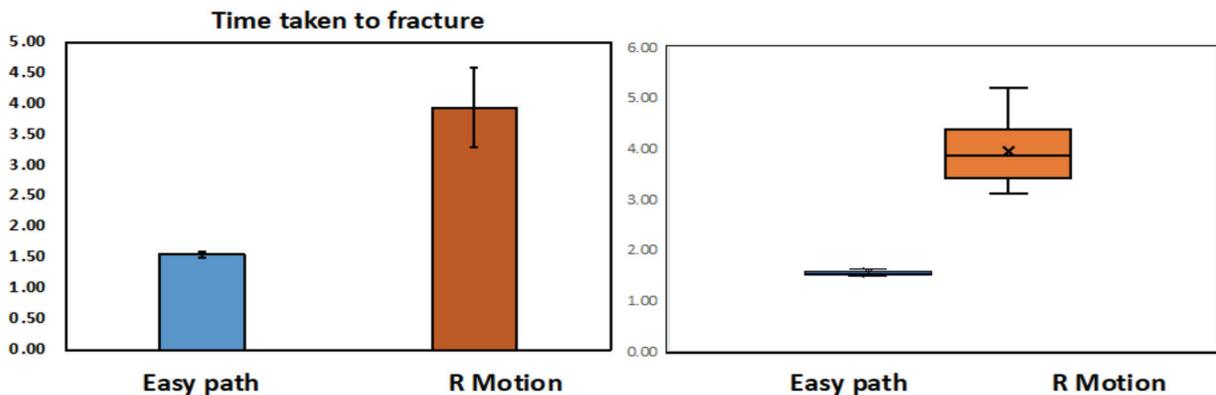
Fig. (2) Bar chart and boxplot presenting the cyclic fatigue in terms of time taken to fractures (seconds).
