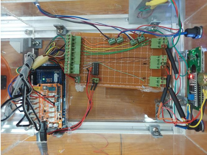
Figure 12: The electrical connection of the whole circuit
