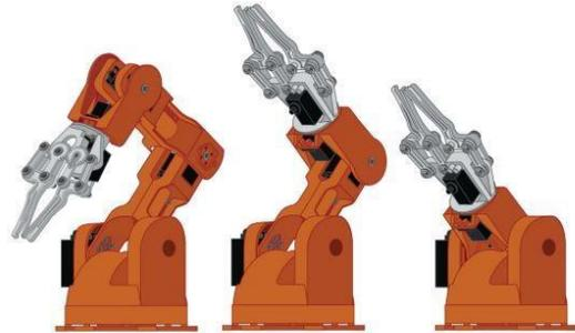
Figure 11: Tinker Kit Braccio Robotic Arm
