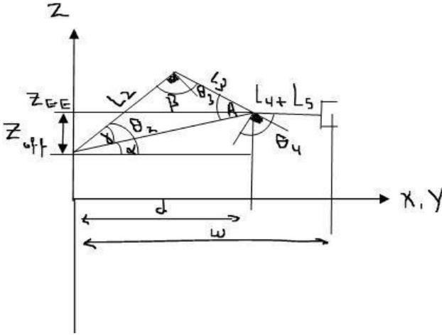
Figure 8: Side view of kinematic diagram
