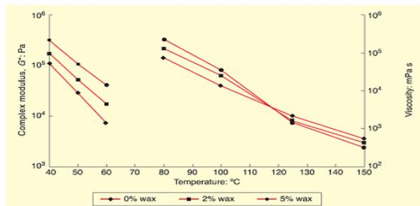
Fig. (6) The effect on the viscosity of a bitumen of adding a selected paraffin wax.
