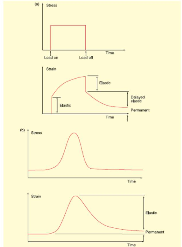
Fig. (5) Visco-elastic responses of asphalt under (a) a static load and (b) a moving wheel load
