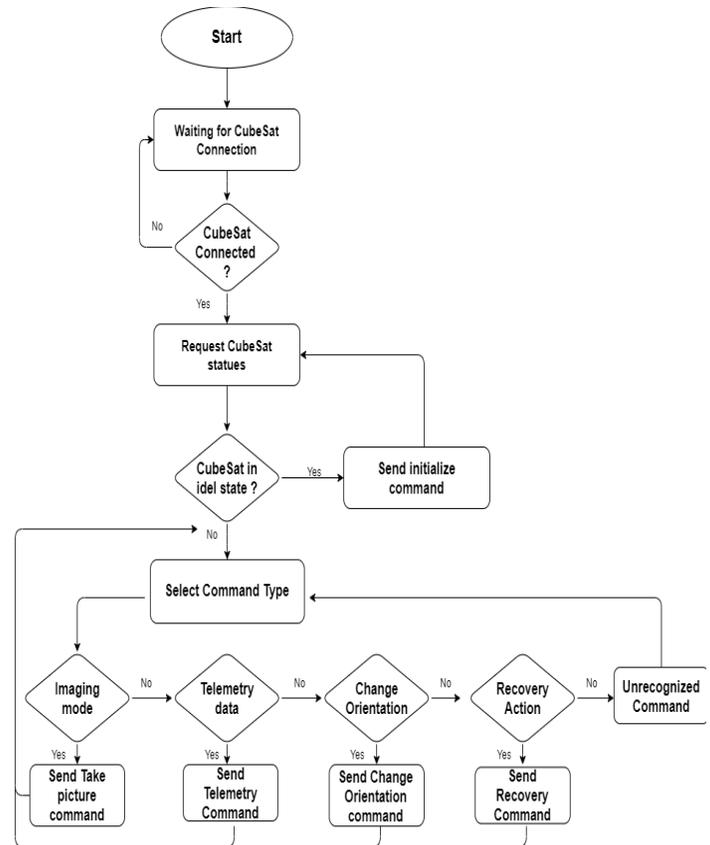
Figure IV.VII (Software Code Flowchart)
