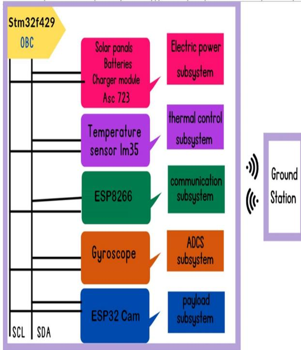
Figure IV (CubeSat lite OBC Architecture)
