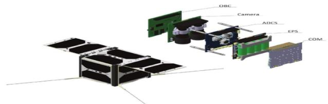
Figure II. I (CubeSat Subsystems)
