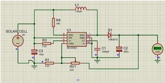
Figure 10 Simulation of boost converter
