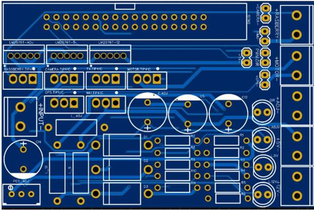
Figure 16 Switching circuit 2D PCB
