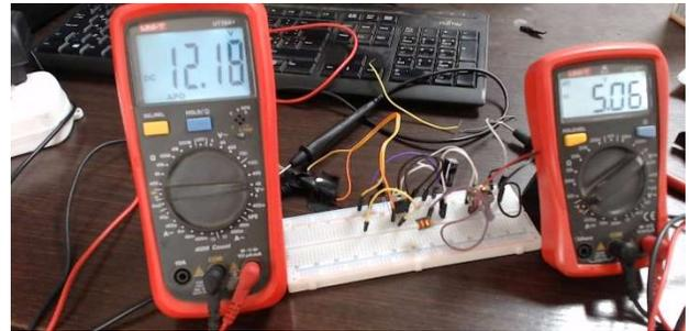
Figure 13 LM2576T-Adj implemented in breadboard
