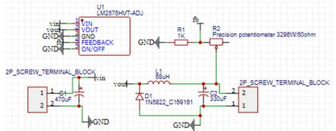
Figure 12 LM2576T-Adj schematic
