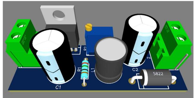
Figure 14 LM2576T-Adj 3D model of PCB
