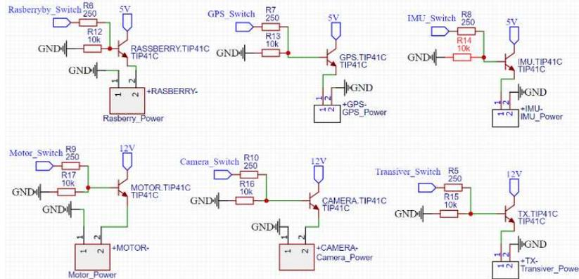
Figure 15 Switching circuit schematic
