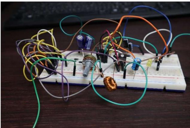
Figure 11 Boost converter implemented in breadboard
