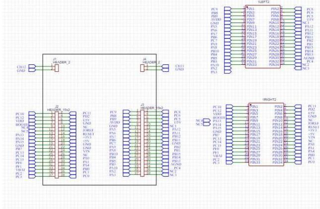
Figure 22 Secondary PCB contains STM Schematic
