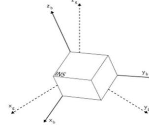
Fig. 2 The body and global frames of reference
