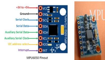
Fig. 3 MPU pinout and configuration
