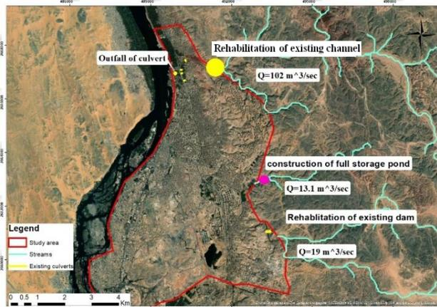
Fig. 18 Conceptual Design of Alternative 02
