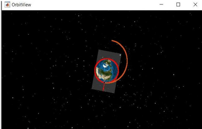
In spaceflight, an orbital maneuver (otherwise known as a burn) is the use of propulsion systems to change the orbit of a spacecraft. You can add it in satellite velocity direction or in normal or in binormal. So you can do it in same Orbit plan or Change Orbit plan.
