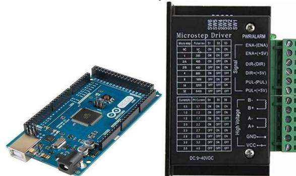
Fig. 10 Arduino Mega 2560 and Stepper Driver TP 6600
