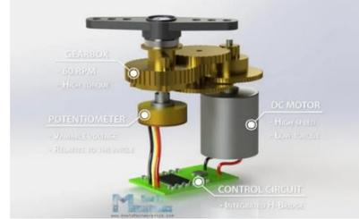
Fig. 15 Servo motor control loop structure
