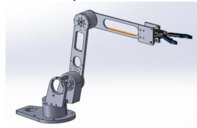
Fig. 5 Robotic arm assembly
