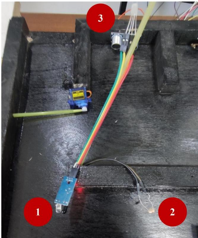
Fig 7 Smart Lighting System (1) IR Sensors, (2) LDR Sensor and (3) LED.
