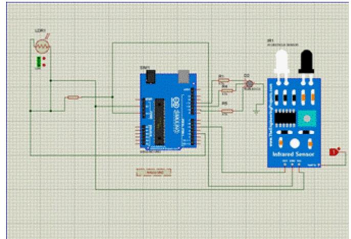
Fig 6 Connection of the smart lightening system.
