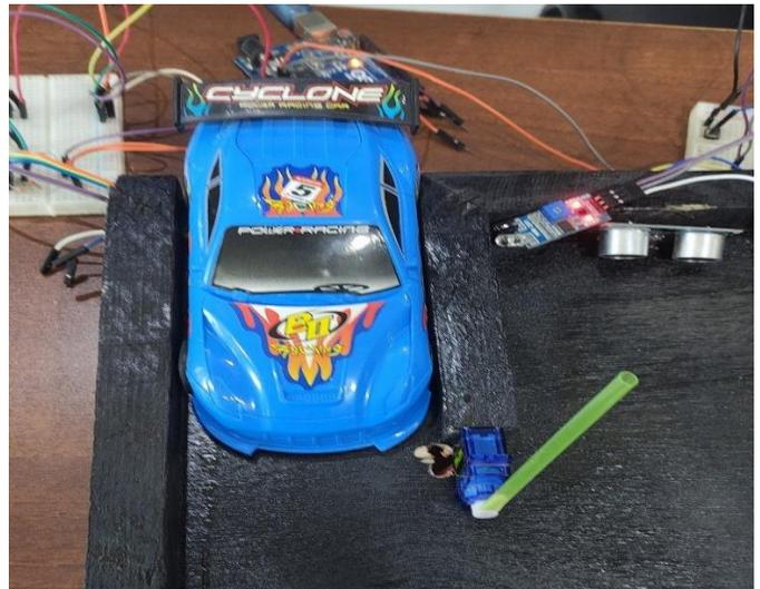
Fig 2 Car detected by IR sensor when entering the gate
