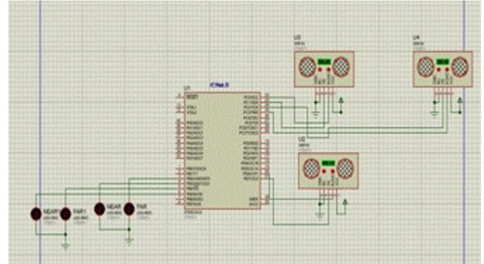
Fig 5 Connection of the ultrasonic sensors and the AVR.
