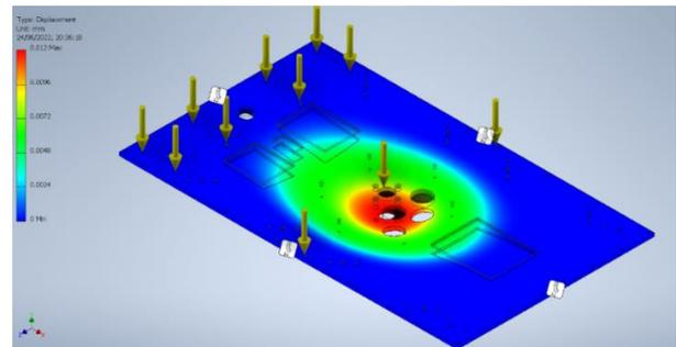
**Fig. 6: Vehicle base stress analysis against deflection**
