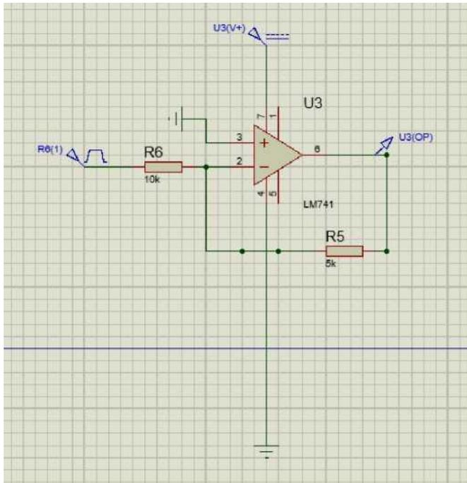
Fig. 7. general schematic of the inverting operational amplifier with the gain amplitude with the feedback resistor  $V_i \left(1 + \frac{R_1}{R_2}\right) (1 + \dots)$
