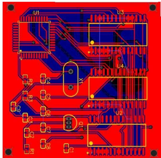
Fig. 9. the routing file
