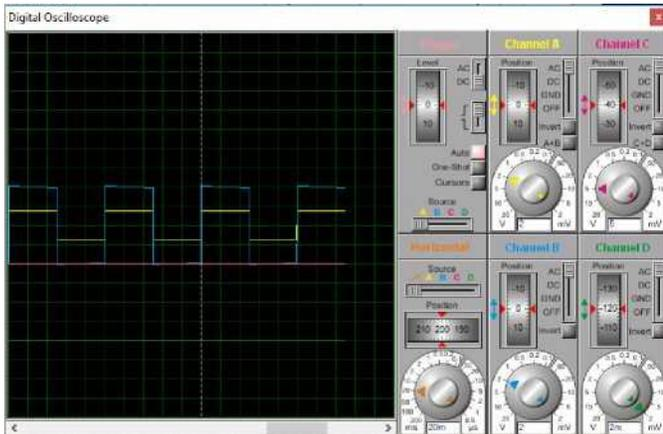
Fig. 3. shows the output of the gain amplifier with the gain amplifier (G=11).
