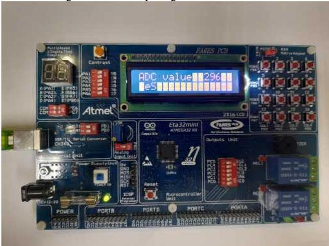
Fig. 11. Monitoring the ADC output using Fares PCB based on Atmel code
