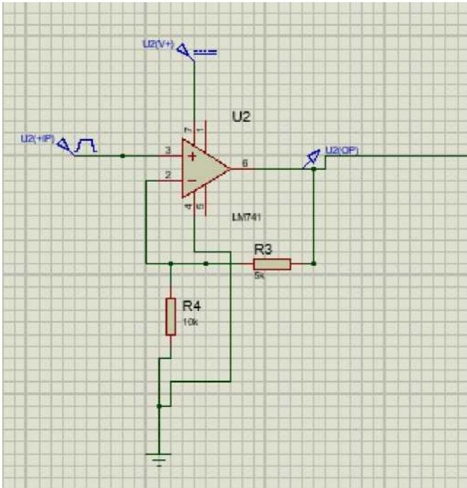
Fig. 2. the Pre-amplifier circuit
