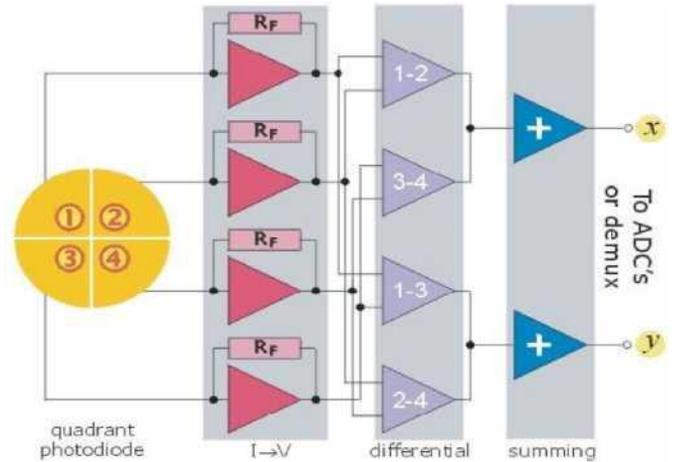
Fig. 1. the general block diagram of the four quadrant detector with processing circuit for laser position determination/
