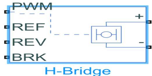
IS used to represent h-bridge motor driver which controls the power input to the motor according to the load requirements. Controlled PWM voltage produce a pulse width modulated signal to control voltage fed to H\_ bridge as per requirement. a solver configuration block specific solver parameter necessary for simulation and is connected to the physical network of the motor controller.
