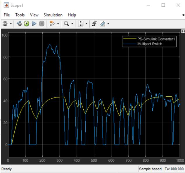
Fig. 4 the first comparison BETWEEN VEHICLE speed and the driving cycle speed
