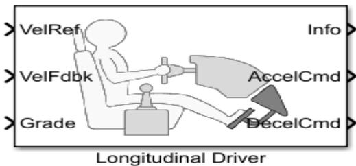
block implements a longitudinal speed tracking controller. Based on reference and feedback velocities, the block generates normalized acceleration and braking commands that can vary from 0 through 1. You can use the block to model the dynamic response of driver or to generate the commands necessary to track a longitudinal driver cycle. Vehicle body
