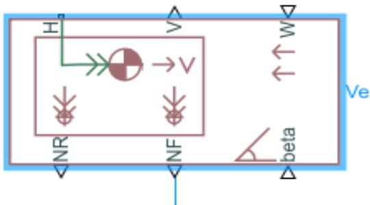
represents a two-axle vehicle body in longitudinal motion. The block accounts for body mass, aerodynamic drag, road incline, and weight distribution between axles due to acceleration and road profile. The vehicle can have the same or a different number of wheels on each axle. Optionally include pitch and suspension dynamics. The vehicle does not move vertically relative to ground
