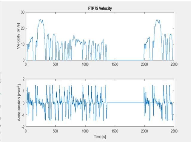
Fig. 2 the velocity and acceleration of ftp\_75 drive cycle
