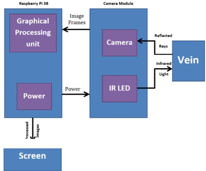
Fig 3 Data/Power Signals Transferred Between the Three Main Layers
