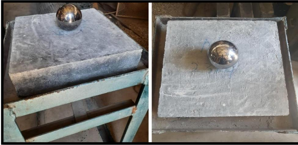
**Figure 4.** Drop weight impact testing.
