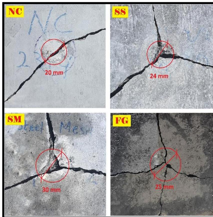
**Figure 9.** Failure mode of different concrete panels.
