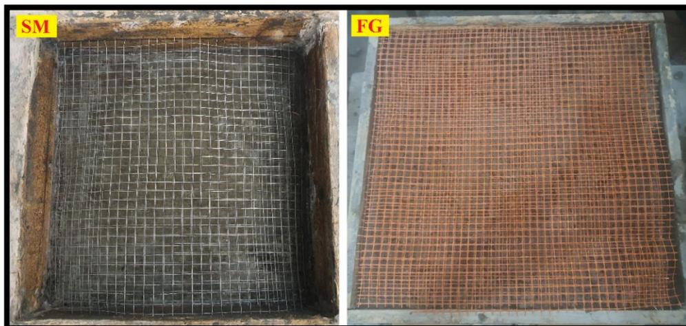
**Figure 2.** Utilizing SM and FG as reinforcement techniques.
