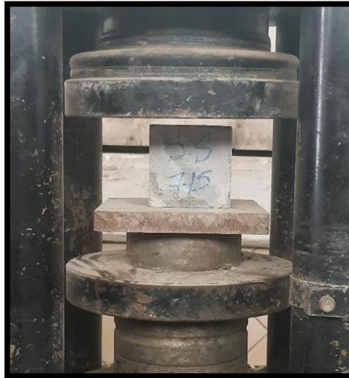
**Figure 3.** Compressive strength test setup.
