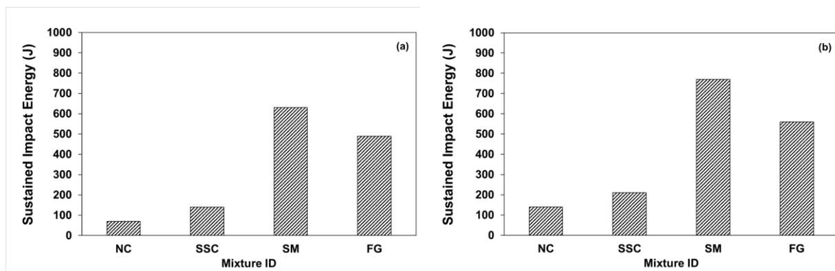
**Figure 7.** Sustained impact energy up to 1<sup>st</sup> crack on; a) upper face and b) lower face.
