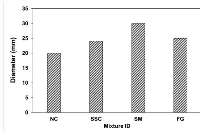
**Figure 6.** Upper face impact diameter of various concrete panels.
