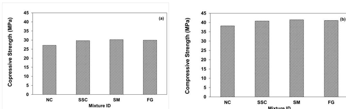
**Figure 5.** The compressive strength of different concrete samples at; a) 7 and b) 28 days.
