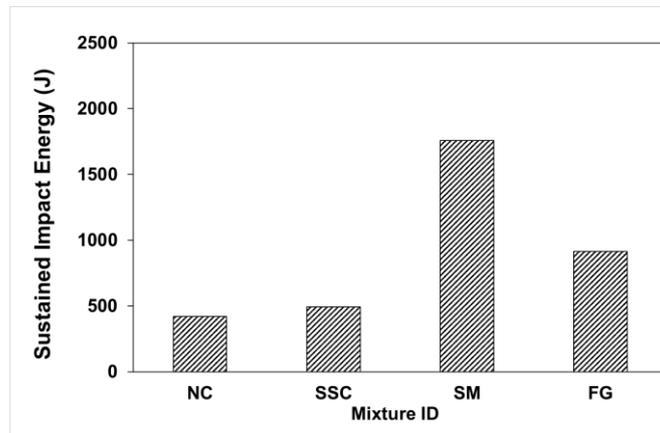
**Figure 8.** Sustained impact energy up to fracture of the various concrete panels.
