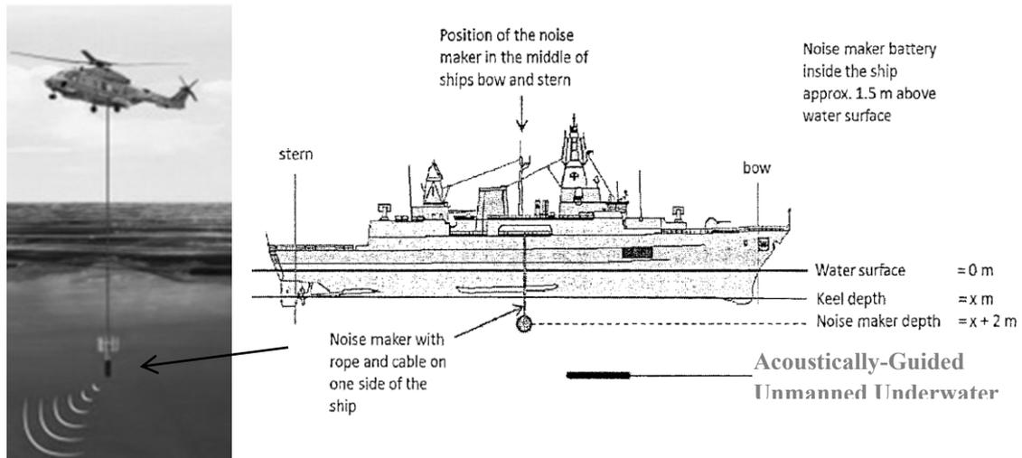
**Figure 1.** Application of NM in testing AGUUV.
