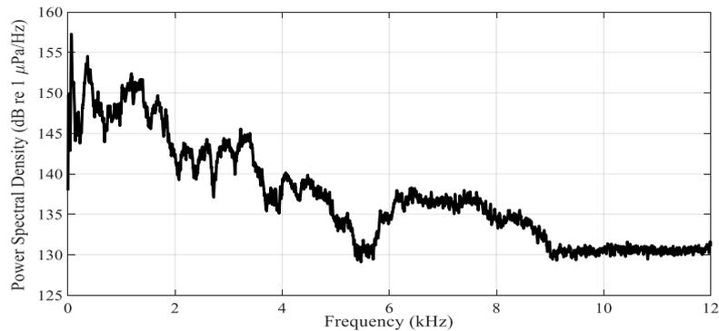
**Figure 4.** PSD of SVN from second example ship
