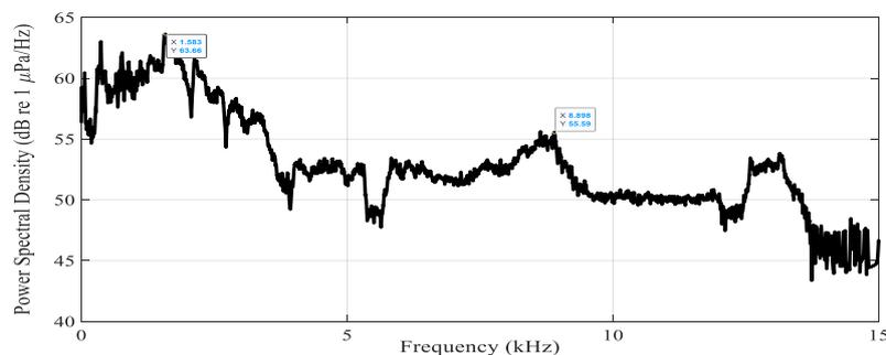
**Figure 2.** AGUUV Noise: PSD of the AGUUV self-noise.
