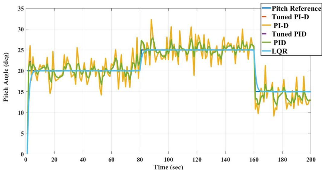
**Figure 4.** Desired pitch angle under the effect of external disturbances and measurement noise.
