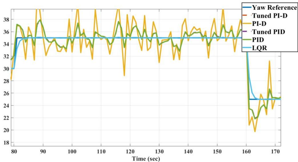
**Figure 7.** Variation of the yaw angle to show the strengthen of the proposed LQR.
