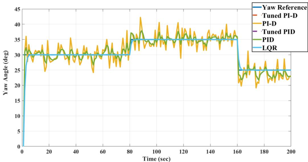
Figure 6. Desired yaw angle performance under the effect of external disturbances and measurement noise.
