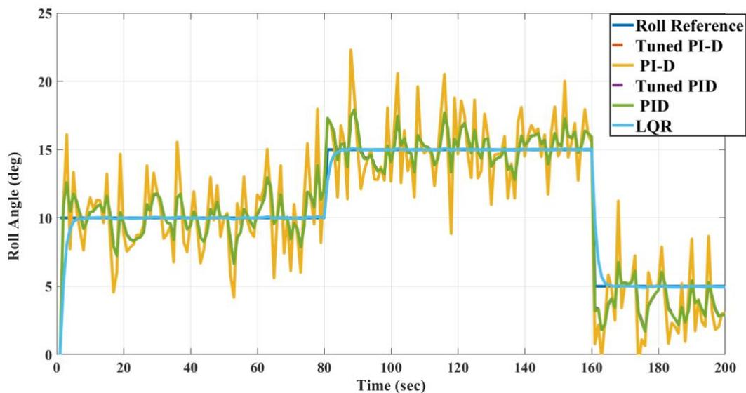
**Figure 2.** Desired angle along the roll axis under the effect of external disturbances and measurement Noise.
