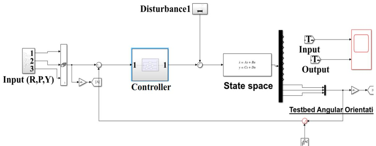
Figure 1. CubeSat Satellite Model affected by External Disturbances and White Noise.
