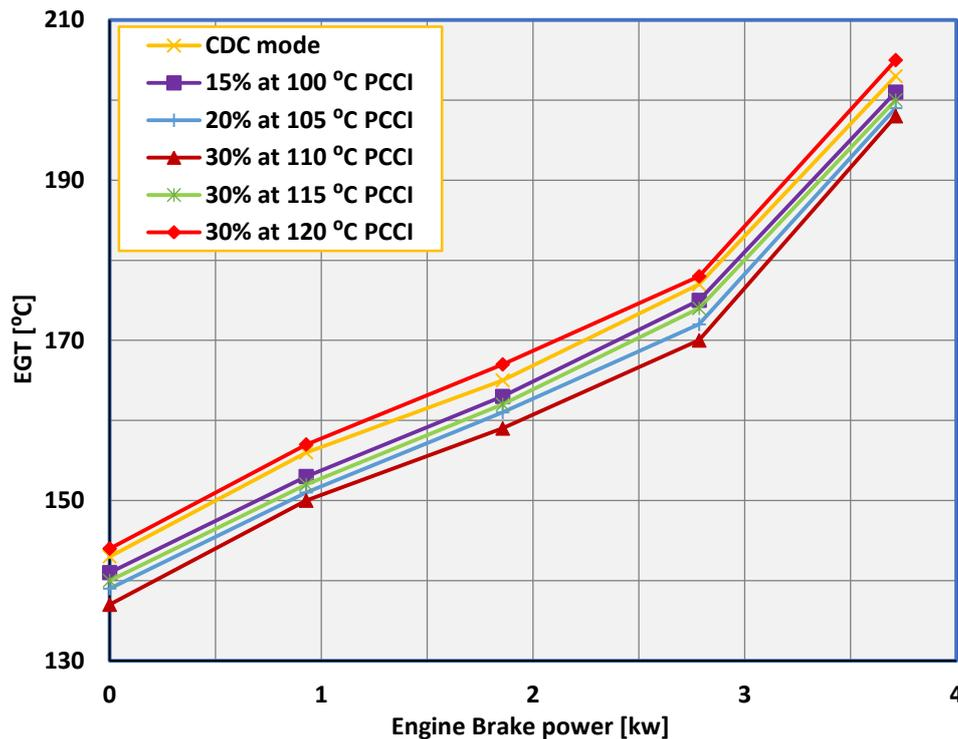
**Figure 8.** Effects of premixed proportion and temperature on PCCI EGT under various loads
