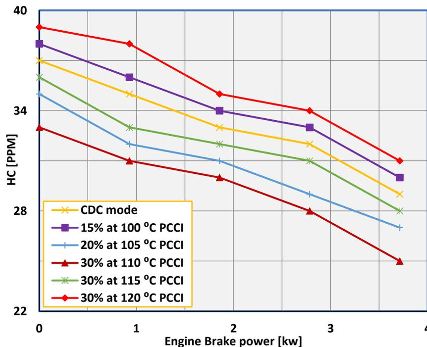
**Figure 12.** Effects of premixed proportion and temperature on PCCI HC emissions under various loads
