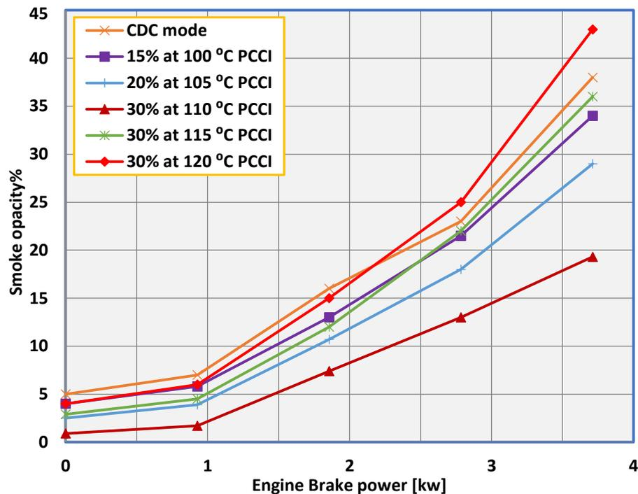
**Figure 13.** Effects of premixed proportion and temperature on PCCI smoke opacity under various loads
