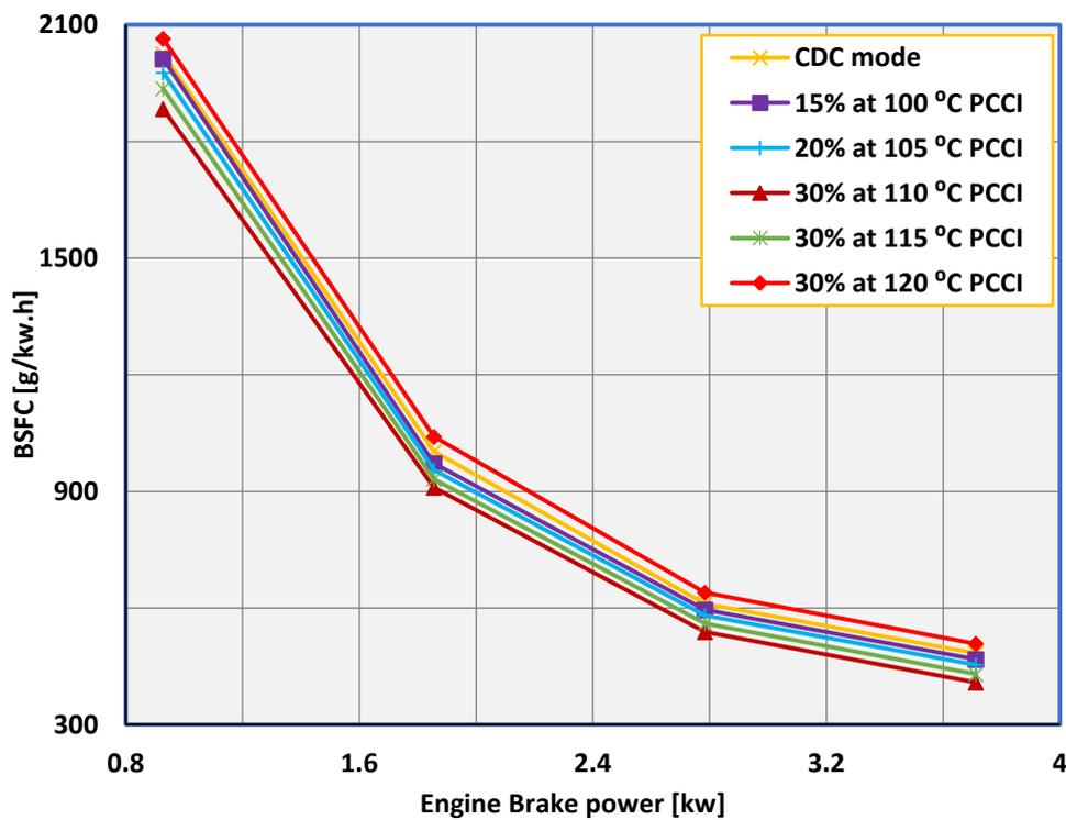
Figure 7. Effects of premixed proportion and temperature on PCCI BSFC under various loads
