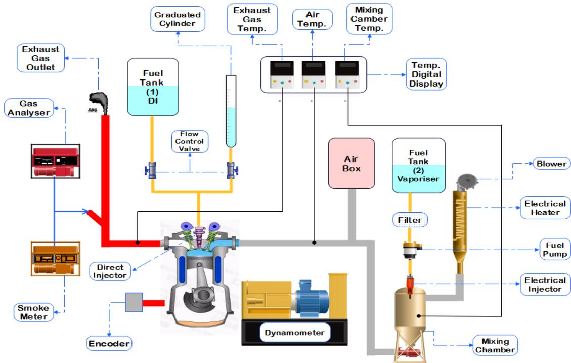
Figure 1. PCCI engine setup schematic diagram with fuel vaporizer.
