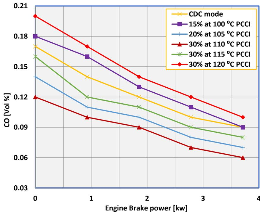
Figure 10. Effects of premixed proportion and temperature on CO emissions of PCCI under various loads
