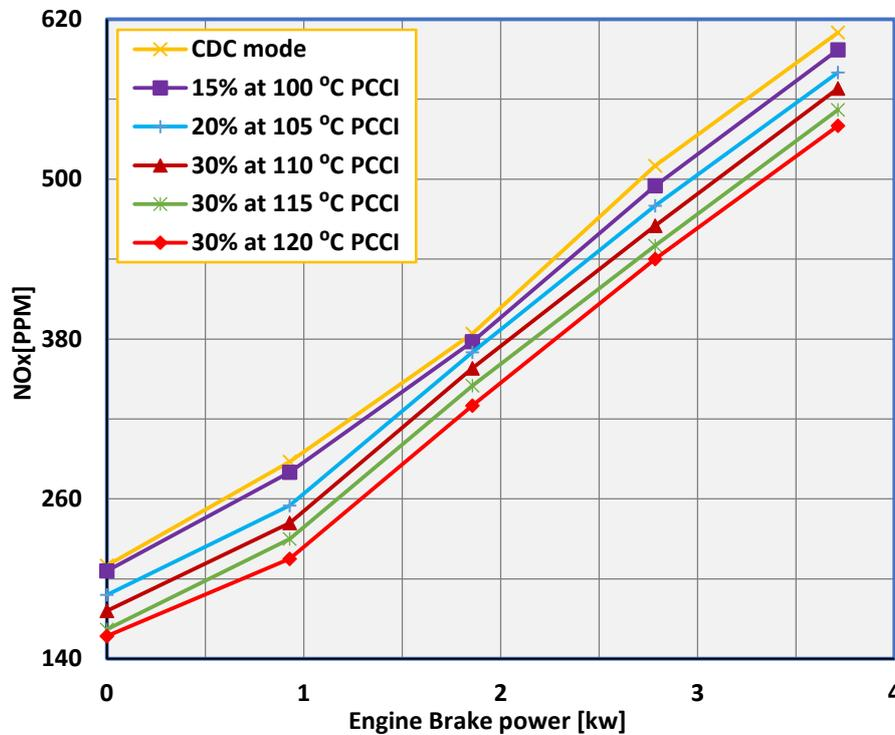
Figure 9. Effects of premixed proportion and temperature on PCCI NO<sub>x</sub> emissions under various loads
