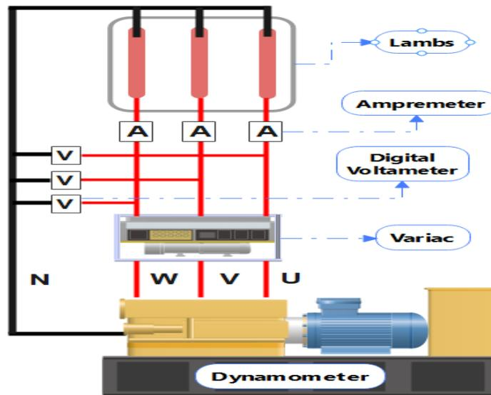
**Figure 3.** Schematic diagram for a load and dynamometer circuit.
