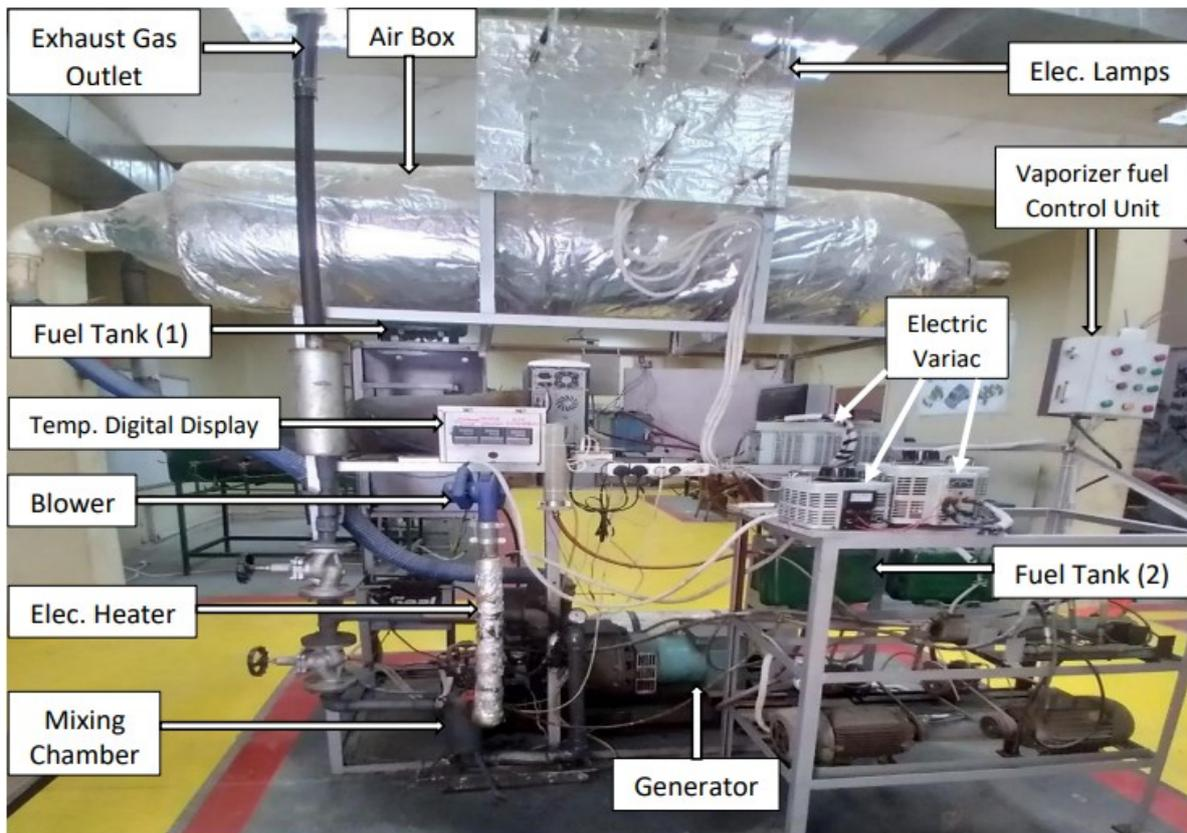
Figure 2. Actual photo of the engine's experimental setup with a fuel vaporizer.
