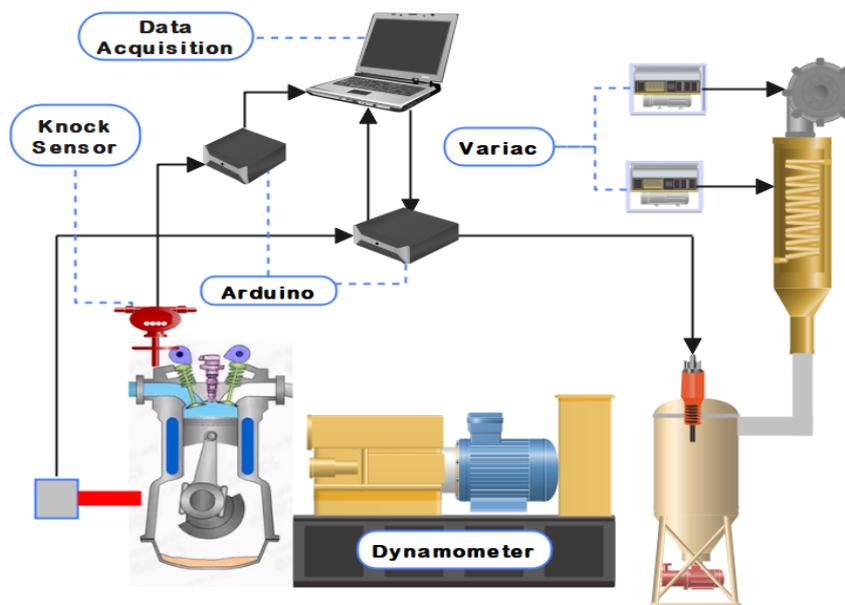
**Figure 4.** Vibration and vaporizer fuel circuit schematic diagram.
