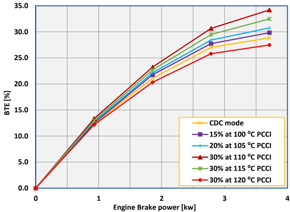
Figure 6. Effects of premixed proportion and temperature on PCCI BTE under various loads
