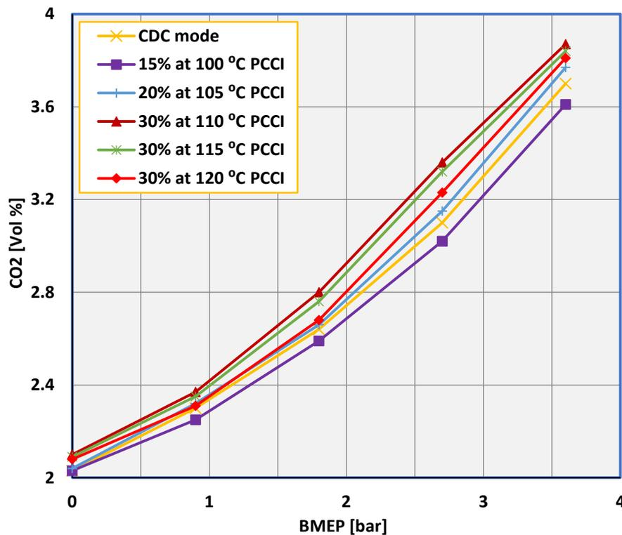
**Figure 11.** Effects of premixed proportion and temperature on PCCI CO<sub>2</sub> emissions under various loads
