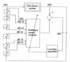
Fig. 4 illustrates the principle of modeling a nonlinear single-input single-output system by learning a neural network.
