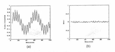
Fig. 5 Time-domain depiction of the neural network output compared with the true nonlinear output (Example 1). a) System response. b) Learning error.
