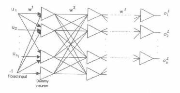
Fig. 2 Multilayer feed-forward neural network.
