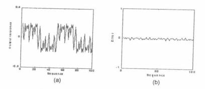
Fig. 8 Time-domain depiction of the neural network output compared with the true nonlinear output (Example 2). a) System response b)Learning error.
