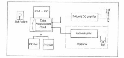
Fig.1. The Nasal Anemometer Configuration
