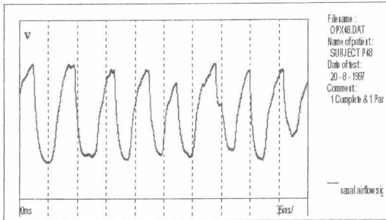
Fig.4. Nasal airflow of abnormal subject with one (nostril) complete and the other is partial obstruction.
