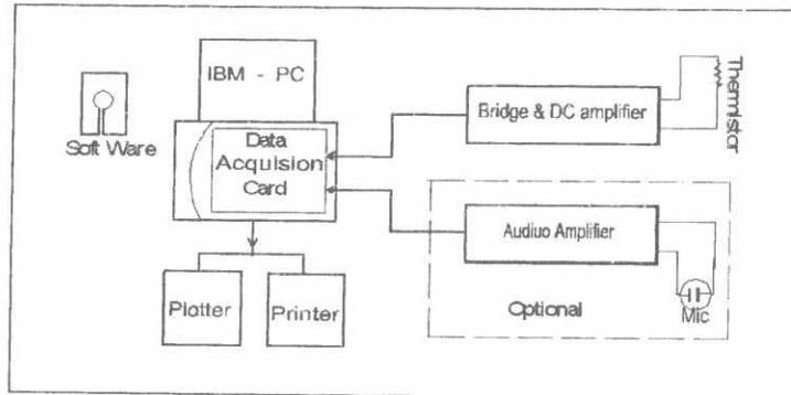
Fig.1. The Nasal Anemometer Configuration
