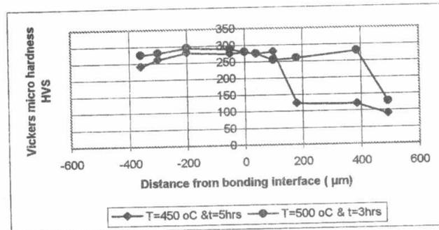
**Fig.17. Vickers Micro hardness values from the interface for a prepared sample using brass as a binding material after aging at P=54MPa, T=450 $^{\circ}\text{C}$  after 5hrs and 500 $^{\circ}\text{C}$  after 3 hrs holding time**
