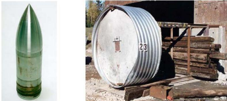
**Fig. 3 The Steel Projectile, Concrete Target used for the Benchmark Test [6].**
