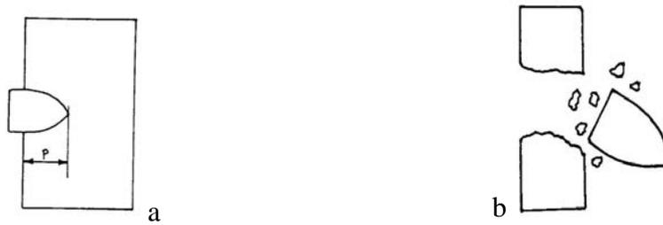
**Fig. 2 Penetration and Perforation Phenomena [5].**
