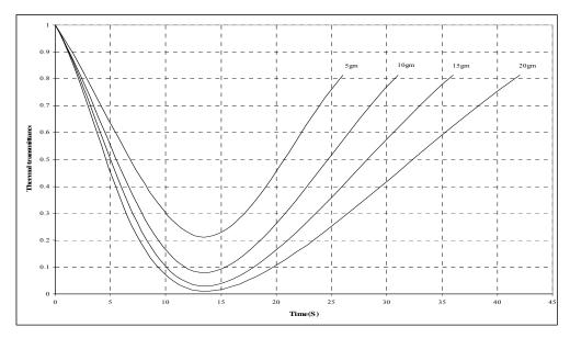
Figure (3.3) Attenuation of infrared radiation emitted from infrared black body radiator at 100°C by cement-dust at relative humidity 35% and ambient temperature 18°C.
