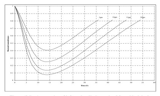
Figure (3.2) Attenuation of infrared radiation emitted from black body radiator at  $100^{\circ}$ C by silica foam at relative humidity 35% and ambient temperature  $18^{\circ}$ C.
