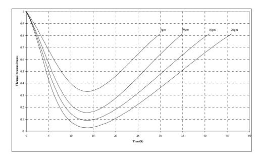
Figure (3.1) Attenuation of infrared radiation emitted from black body radiator at  $100^{\circ}$ C by fly ash at relative humidity 35% and ambient temperature  $18^{\circ}$ C
