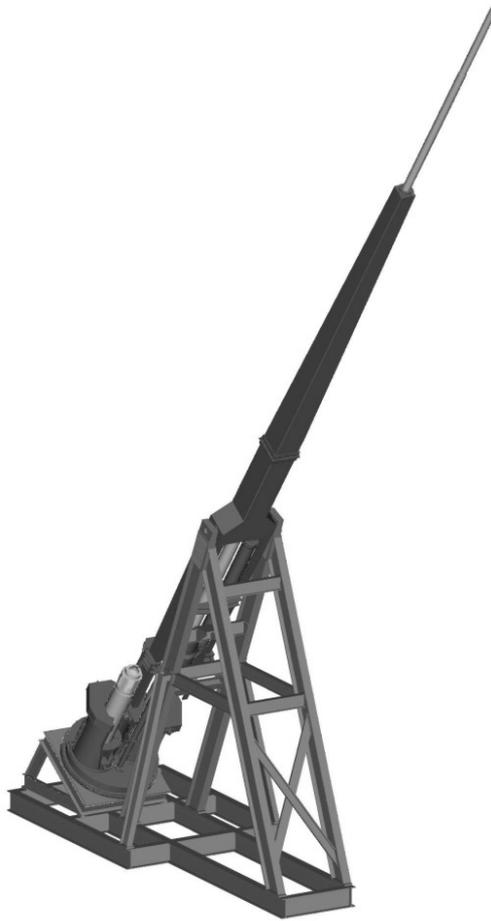
**Figure 4: The Applied Ordnance Technology AOT or XLR Gun<sup>7,8</sup>; AOT Claims It Is Capable of Developing 200 Caliber Barrels**
