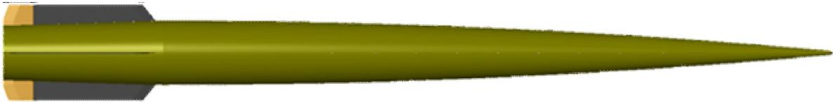
Figure 2: The 5"/12 Calibers, 100 lbs, Dart-Like Barrage Round
