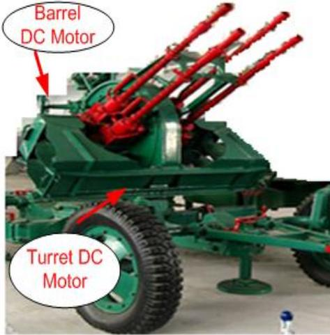
Fig. 1 Real Gun Turret-barrel system
