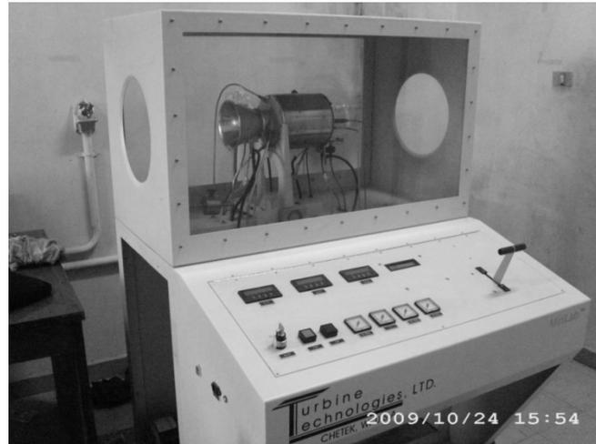
**Fig. 3 SR-30 Test Rig**
