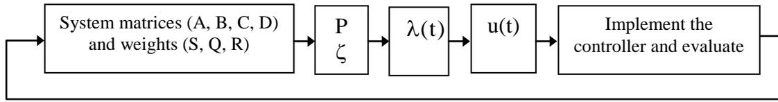
Fig. 7: Sequence of optimal control servomechanism design
