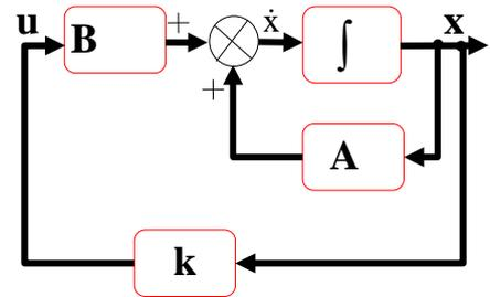
Fig. 1: State Feedback Closed Loop
