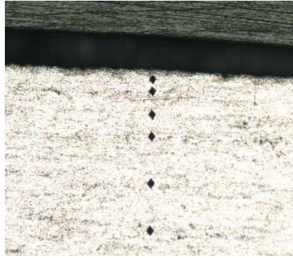
Fig.8 Micro-hardness indentations on SC sample cross-section
