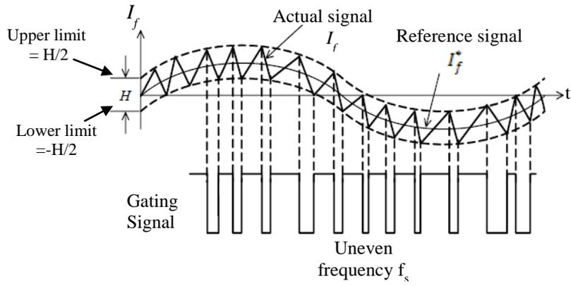
**Fig. 5 Gating signal generation by hysteresis current control technique**
