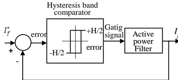
**Fig. 4 Block diagram of current hysteresis control technique**
