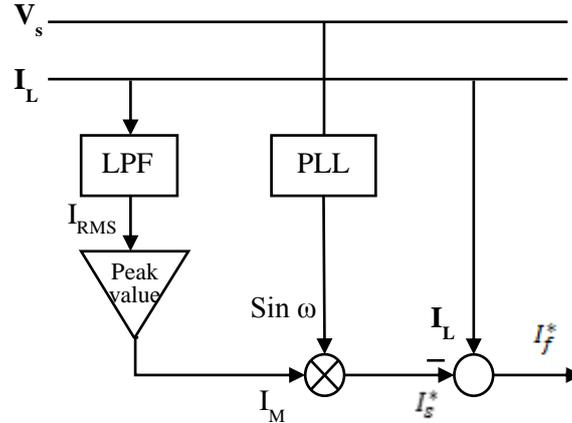
**Fig. 3 Block diagram of the direct testing and calculating method**
