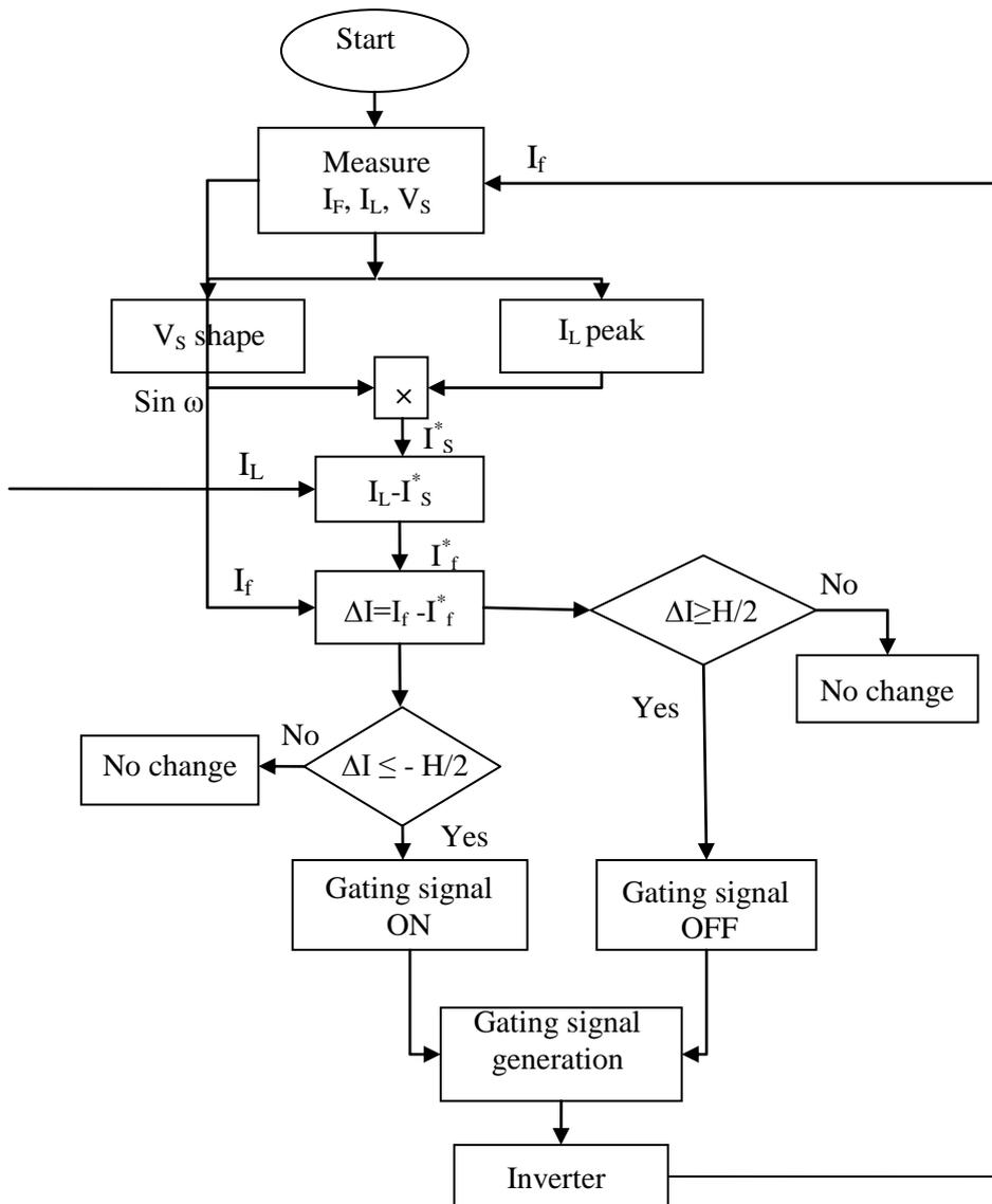
**Fig. 6 Flow chart for the proposed control process**
