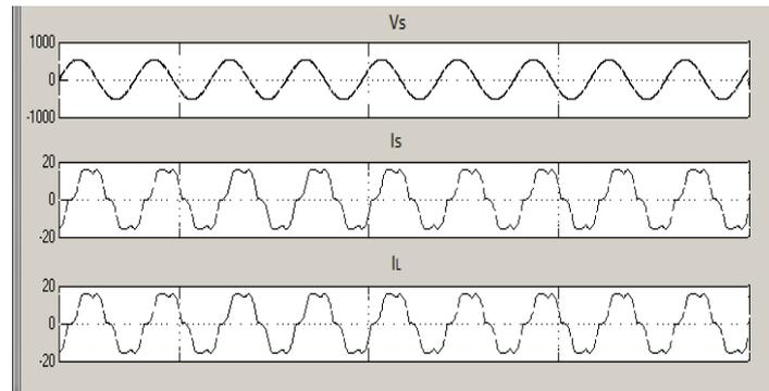
**Fig. 7 simulation results for source voltage ( $V_s$ ), source current ( $I_s$ ) and load current ( $I_L$ ) before compensatin**
