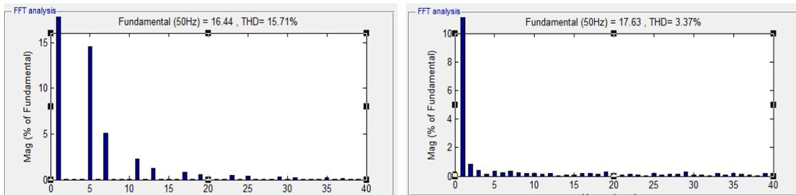
**Fig. 9 (a) Input current harmonic spectrum before compensating (b) Input current harmonic spectrum after compensating**
