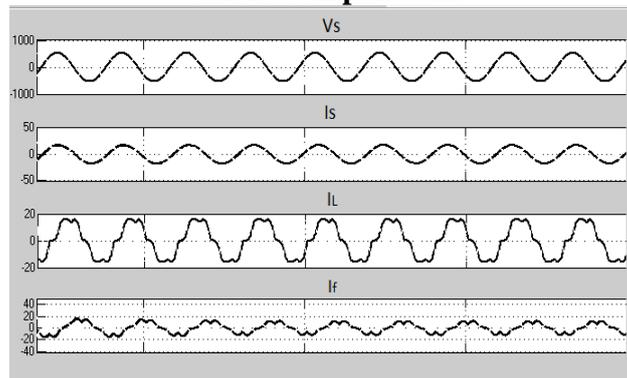
**Fig. 8 waveforms of source voltage, source current, load current and filter current after compensating**
