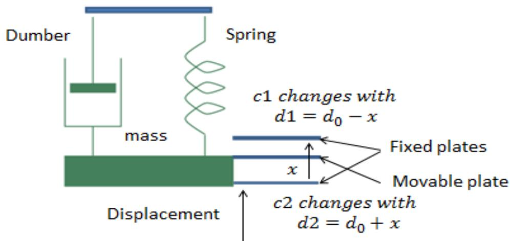
Figure 3 Tilt sensor structure
