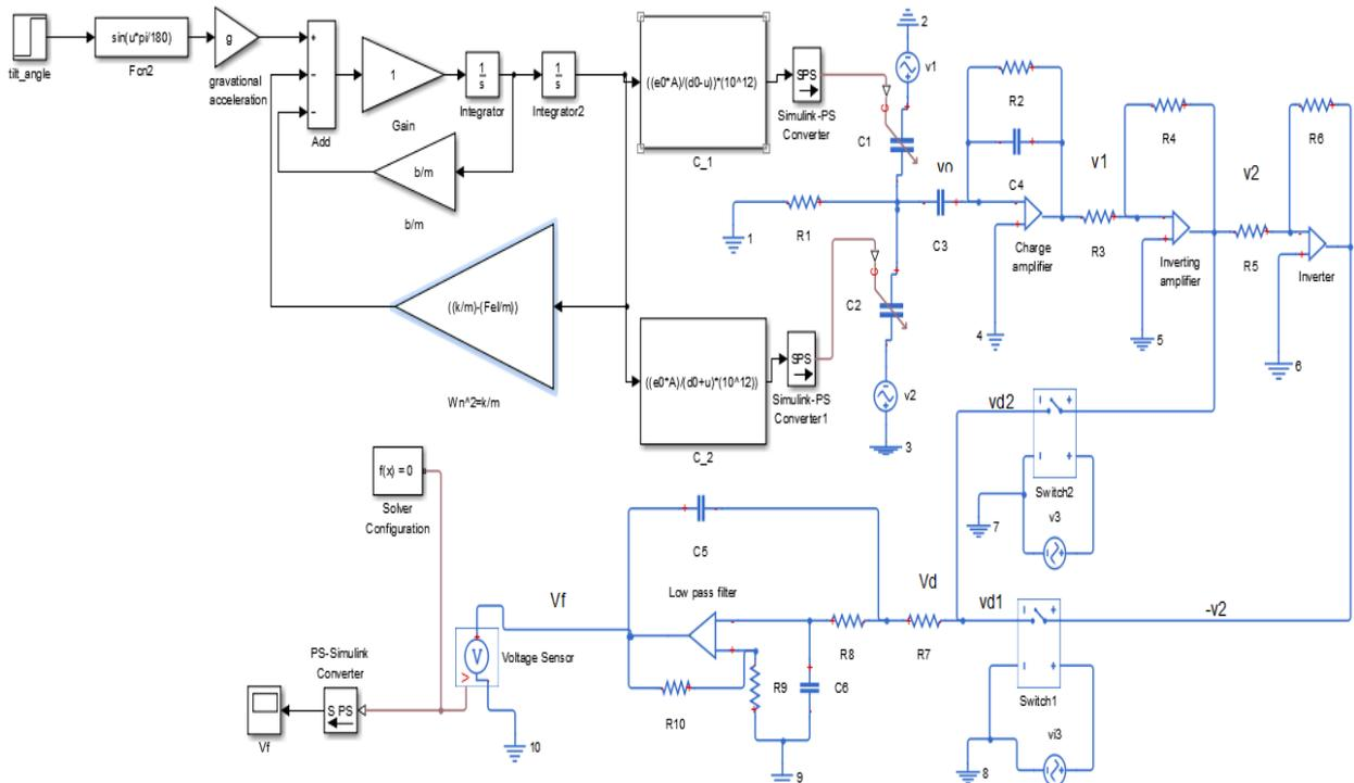
Figure 10 Proposed integrated tilt sensor circuit
