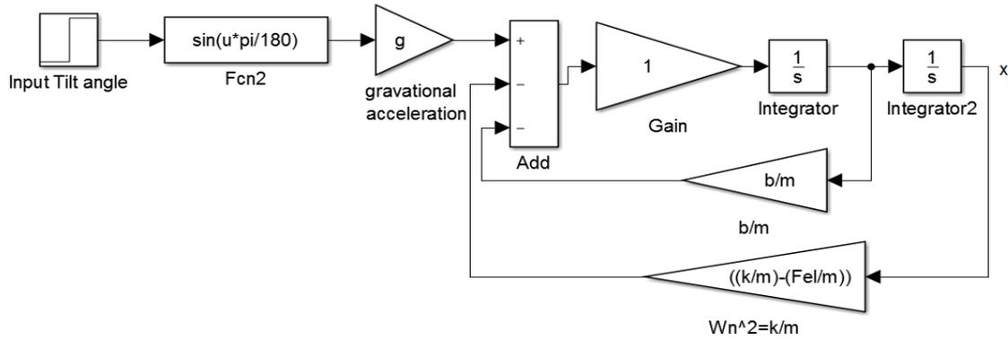
Figure 4 Tilt sensor mechanical part model
