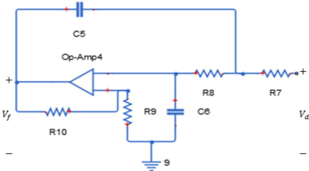
**Figure 9 Low pass filter circuit**
