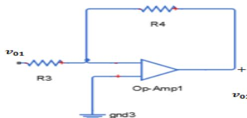
Figure 7 Inverting amplifier
