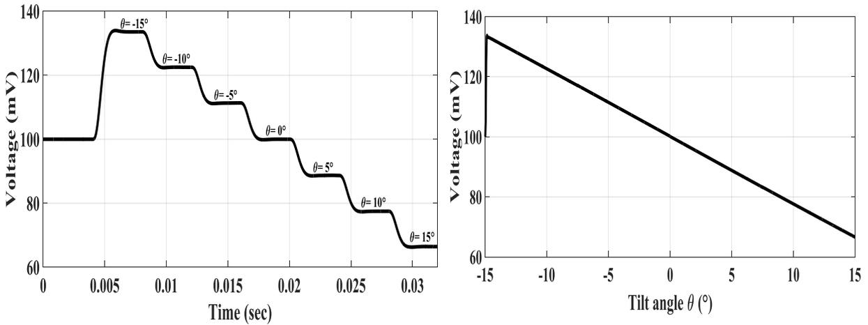
Figure 14 Tilt sensor output voltages after adding noise and bias voltage
