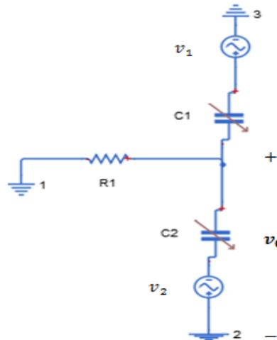
Figure 5 Variable capacitors for tilt sensor
