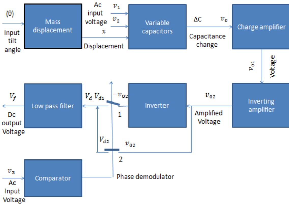
Figure 2 Proposed tilt sensor block diagram
