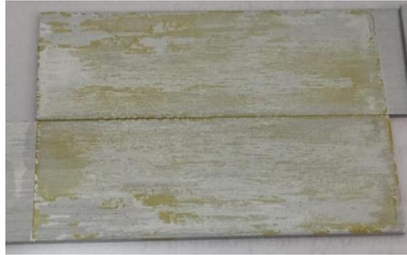
Fig. 6. Sample A3 shear specimen after failure
