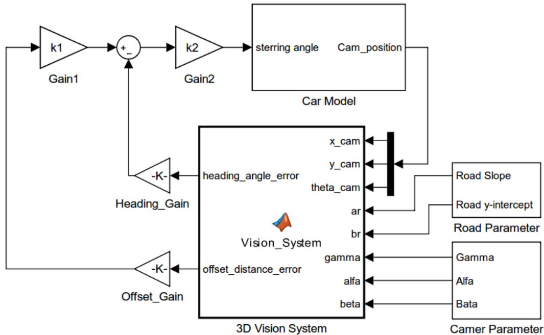
**Fig.23. Simulink Model of 3D Vision Simulation**
