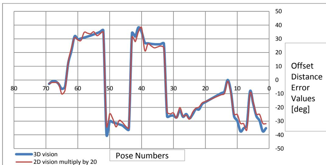
**Fig.21. Offset Distance Error in 3D Vision vs. 2D Vision**
