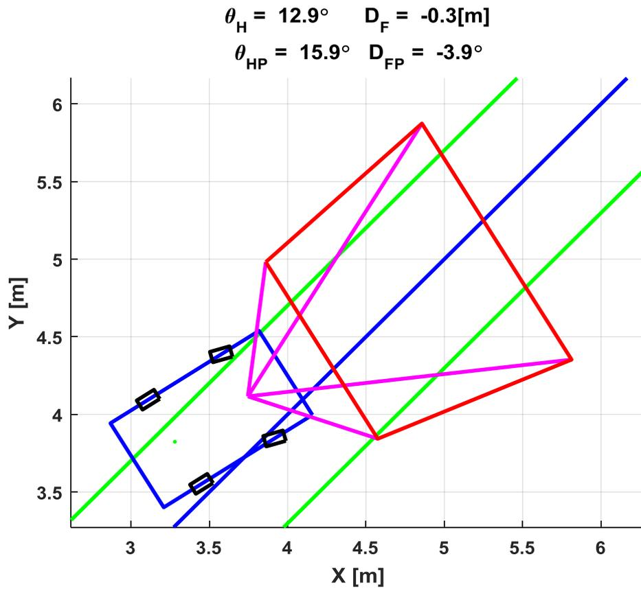
**Fig. 13. Plotting the Vehicle and the Frustum w.r.t Road using MATLAB**
