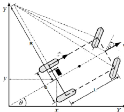
**Fig.5. Kinematic model**
