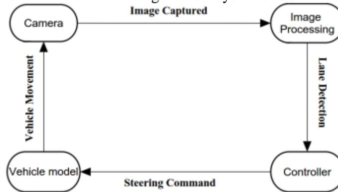
**Fig.4. Subsystems of a Vision-Based Autonomous Vehicle**
