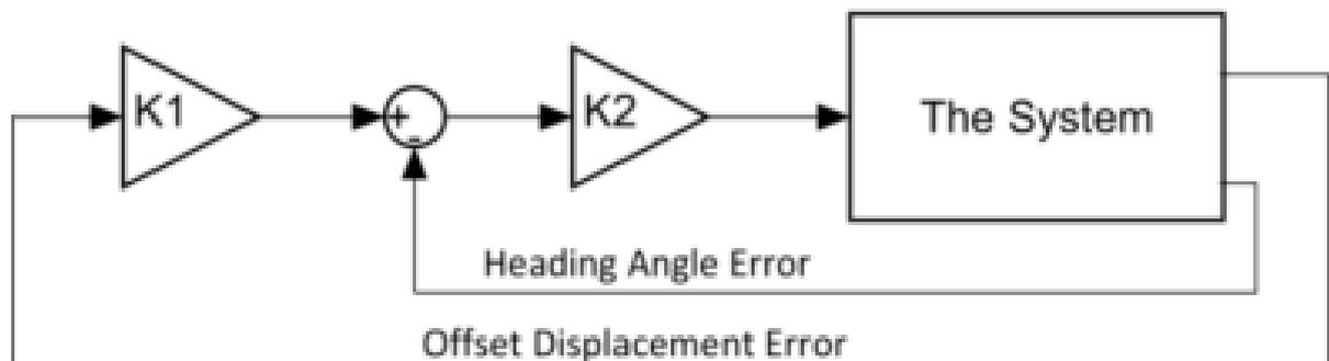
**Fig.16. Successive Loop Closure Diagram**
