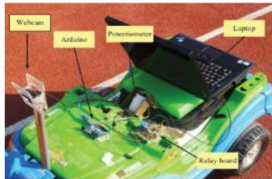
**Fig.3. Experimental Platform Description [3]**
