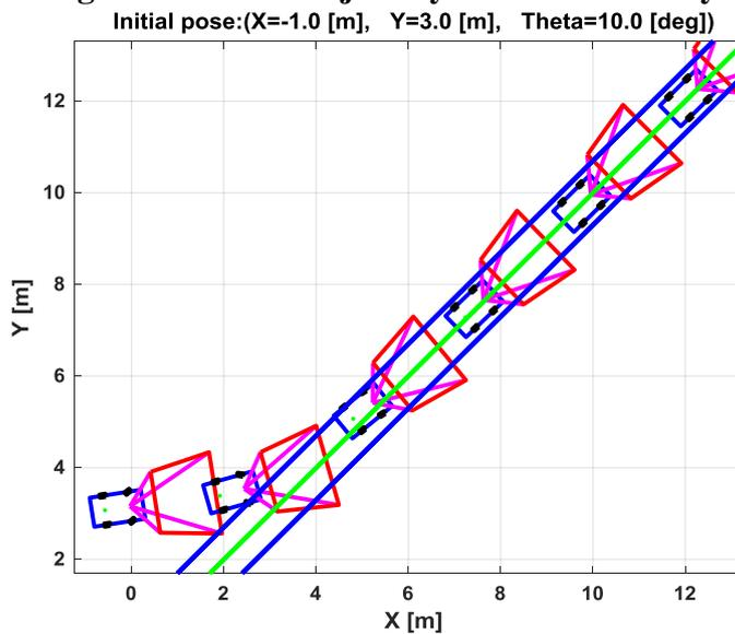
**Fig. 29. Vehicle trajectory with vehicle and frustum**
