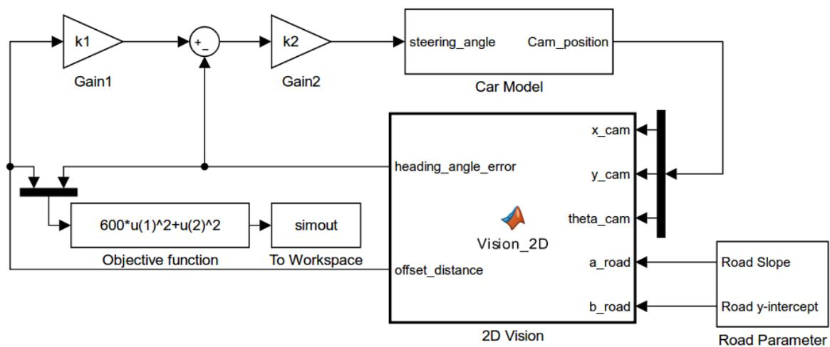
Fig.22. Simulink Model of 2D Vision Simulation
