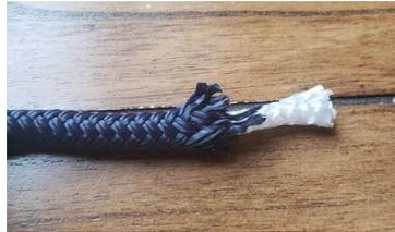
Figure (10) Double braided rope construction.
