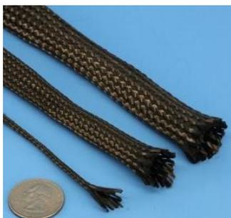
figure (50) (CNT) fiber Rope.
