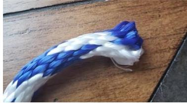
Figure (9) single braided rope construction.
